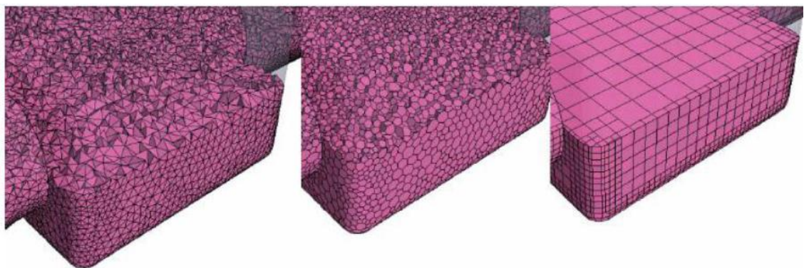
Fig.3.7 Three types of volume meshing; left: tetrahedral, middle: polyhedral, right: trimmer.
