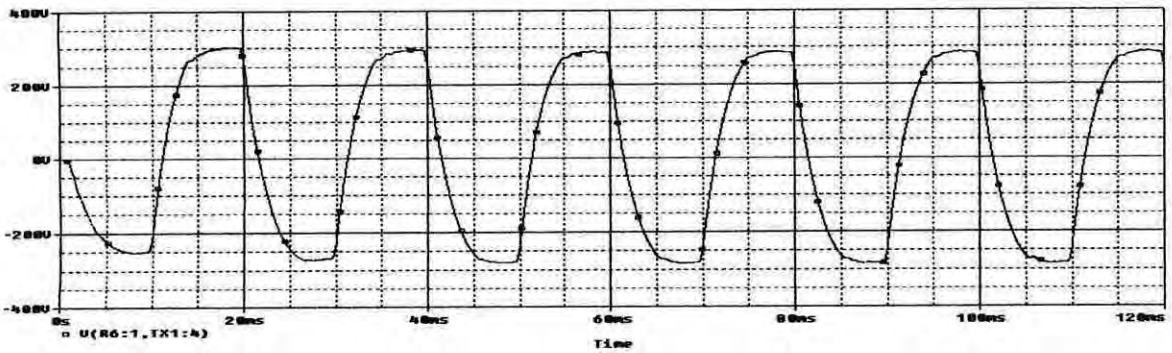
Fig 2.48: Output of modified Ćuk Regulator fed Resonant Inverter (Practical BJT switch implementation)
