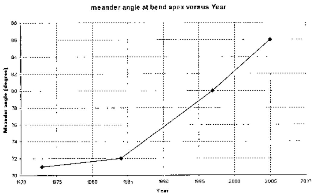
**Figure 2.6: Meander angle at cross over in different years.**
