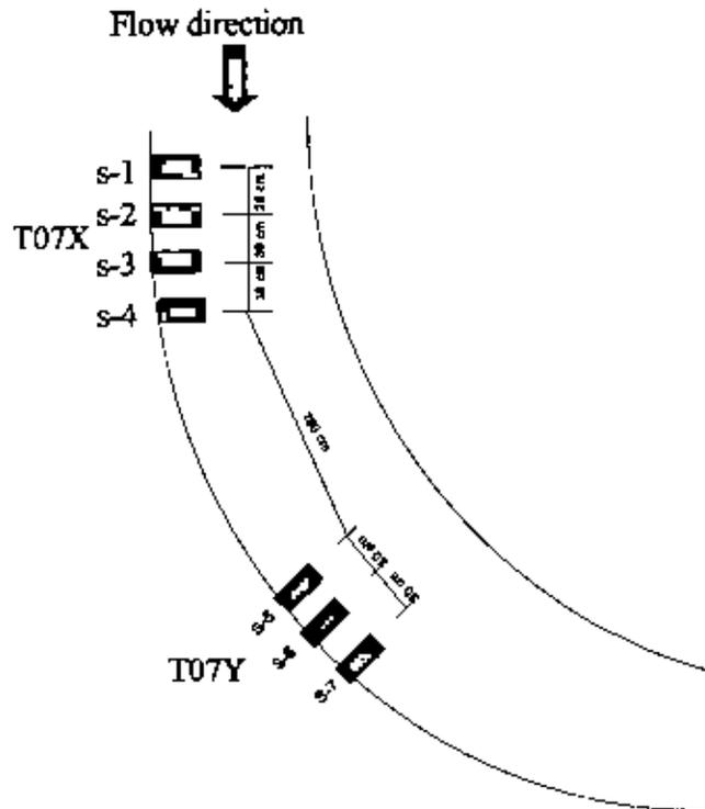
Figure 6.4: Physical set up for T07 (not in scale)
