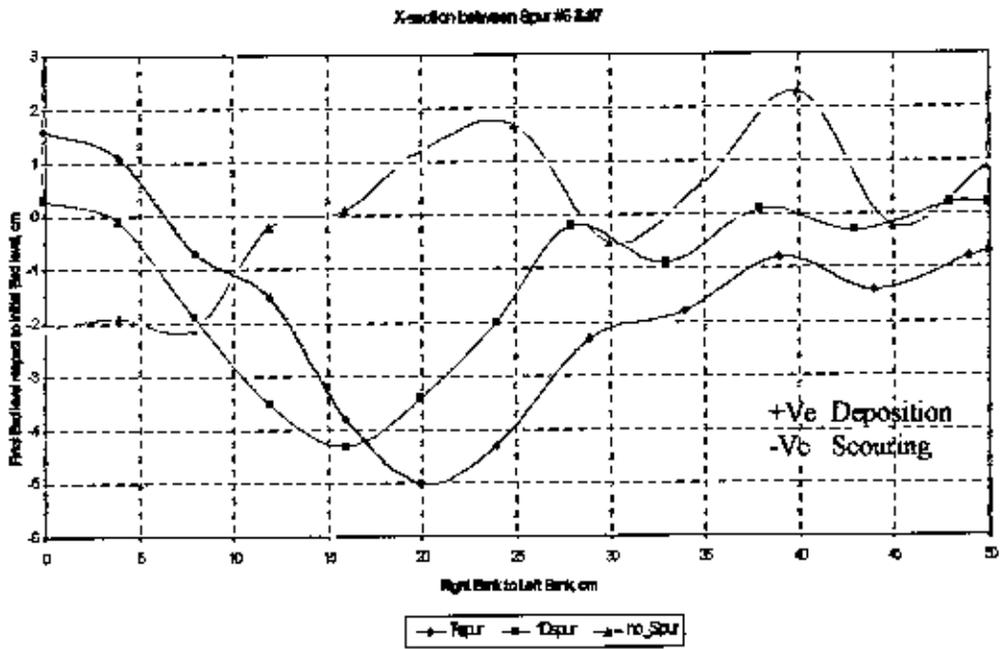
**Figure A5: Cross sections in between spur #6 and #7**
