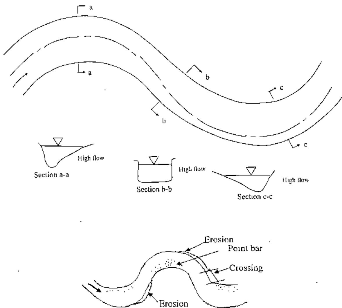
**Figure 3.1: Meandering process at bends**
