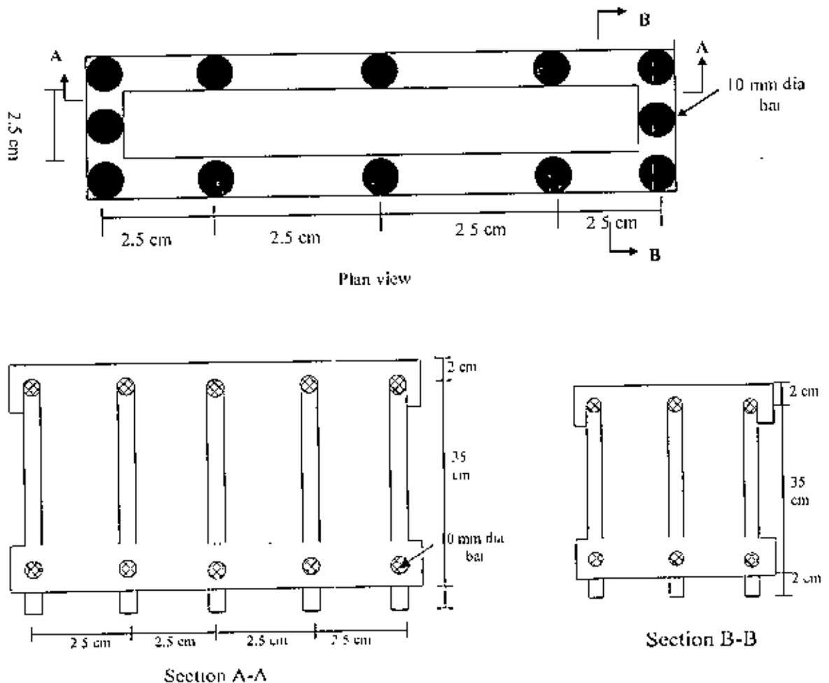
**Figure 6.2: Detail of permeable structures**
