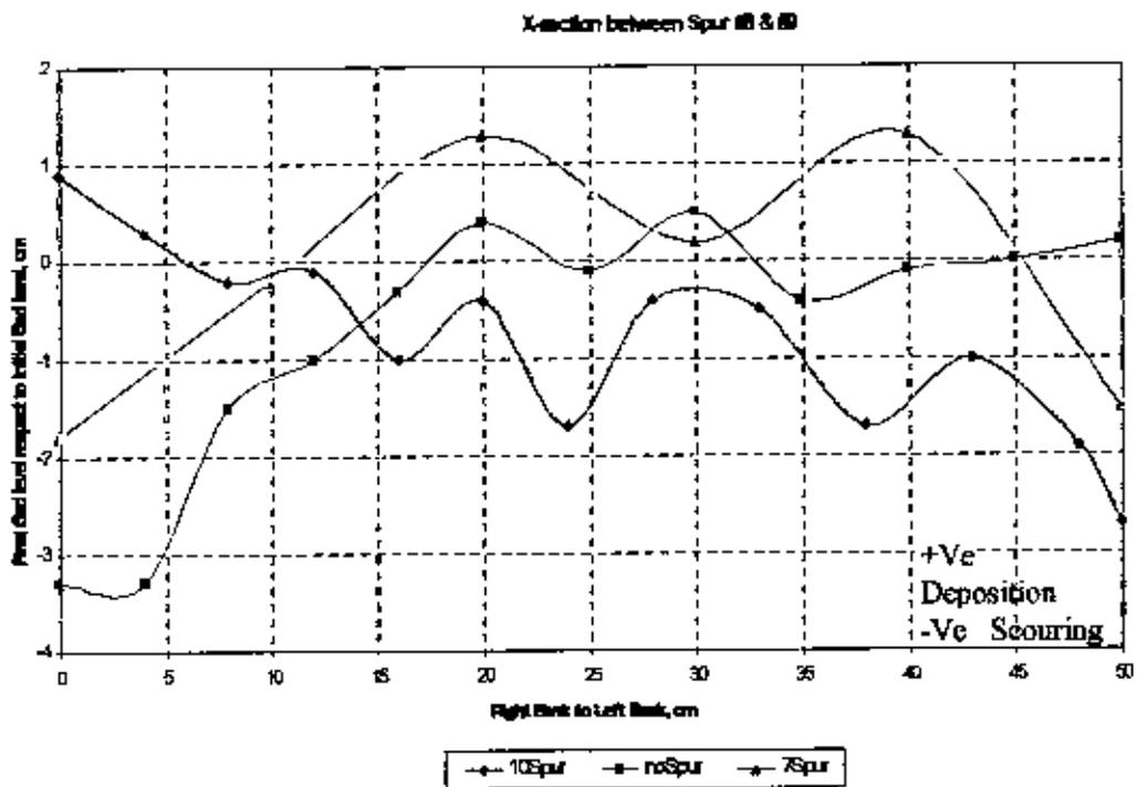
**Figure A8: Cross sections in between spur #8 and #9**
