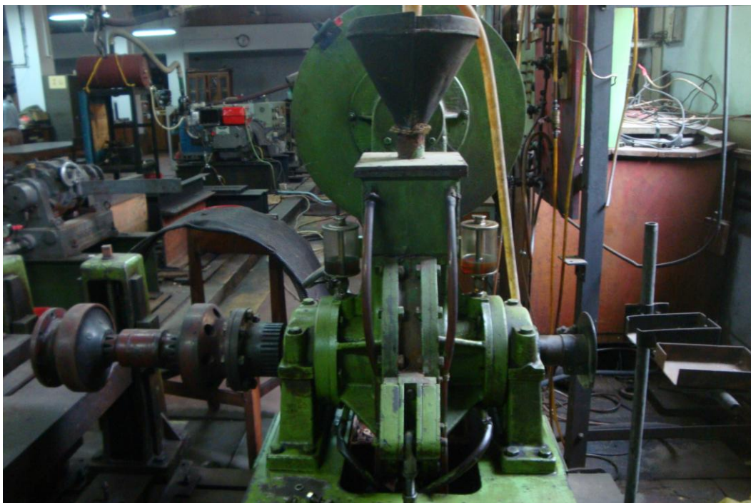
Fig. 4.2: Picture of the water brake type dynamometer, model no. AN3e
