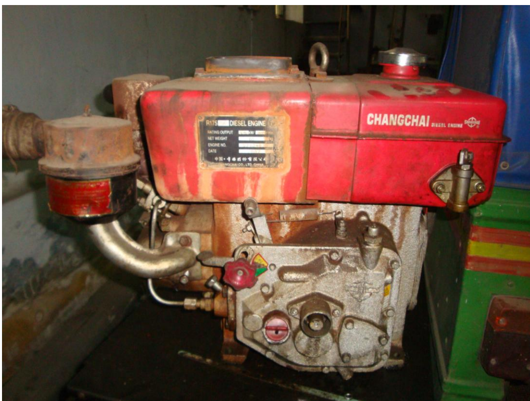
Fig. 4.3: Picture of the diesel engine model R175A
