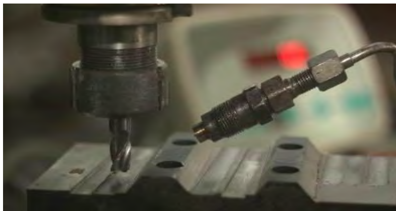
Fig.2.10 Photographic view of Nozzle Injector during milling process
