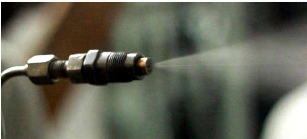
Fig.2.7 Photographic view of spray pattern of the cutting fluid
