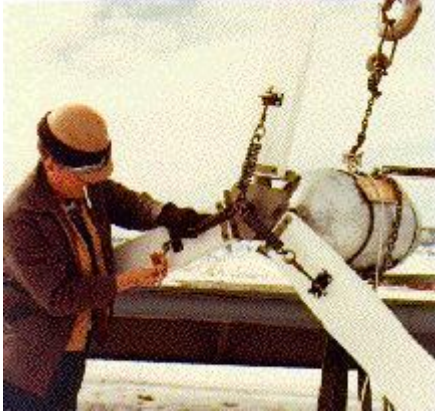
Figure 7. M.L. Jacobs adjusting the spring-actuated pitch change mechanism on a Jacobs Wind-electric in 1977.
