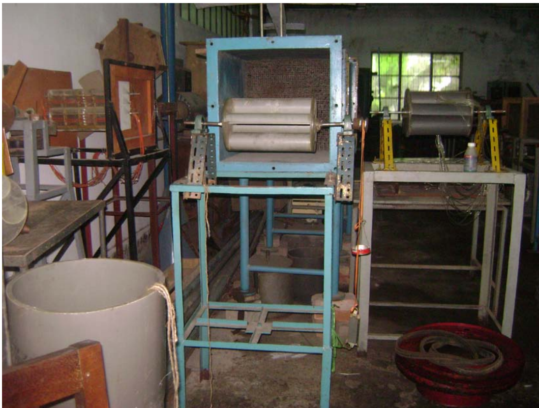
Figure 5. 6: Set – up of the Experiment ( 6 Bladed Vane Type Rotor )
