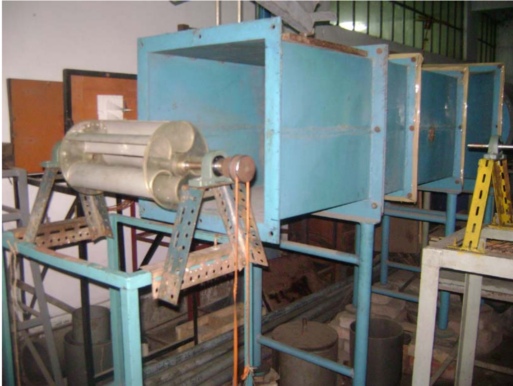
Figure 5. 5: Set – up of the Experiment ( 5 Bladed Vane Type Rotor )
