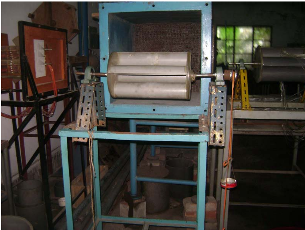
Figure 5. 4: Set – up of the Experiment ( 4 Bladed Vane Type Rotor )
