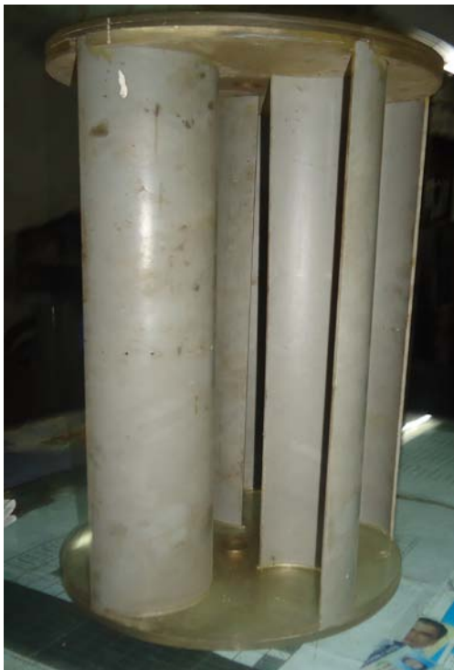
Figure 5. 12: Constructional Details of 5 Bladed Vertical Axis Vane Type Rotor
