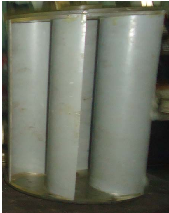
Figure 5. 13: Constructional Details of 6 Bladed Vertical Axis Vane Type Rotor
