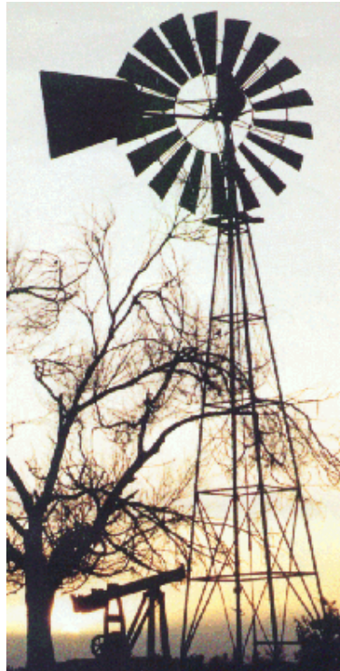
Figure 2. 2: Windmill for water pumping
