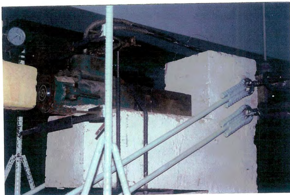
Fig.: 3.14 Hydraulic jack mounted on the cantilever portion of the reaction frame.
