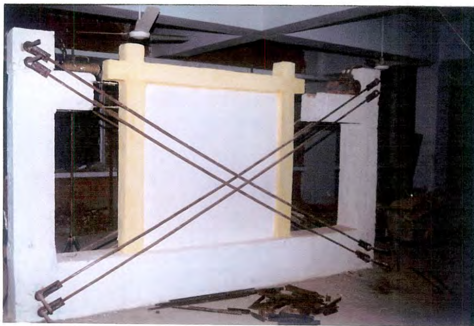
Fig.: 3.7 Test frame with diagonal tie rods attached.
