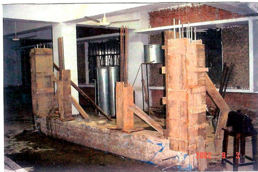
Fig.: 3.10 Construction of the test rig mid way through the casting.
