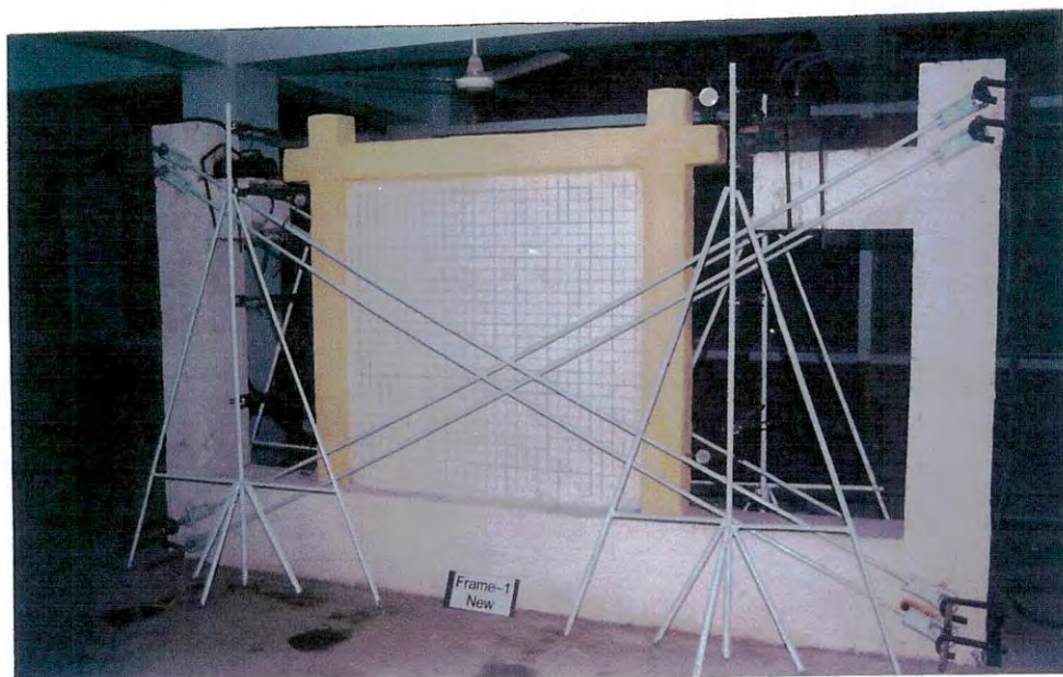
Fig: 3.13 Test setup with mounting frame to mount dial gauges.
