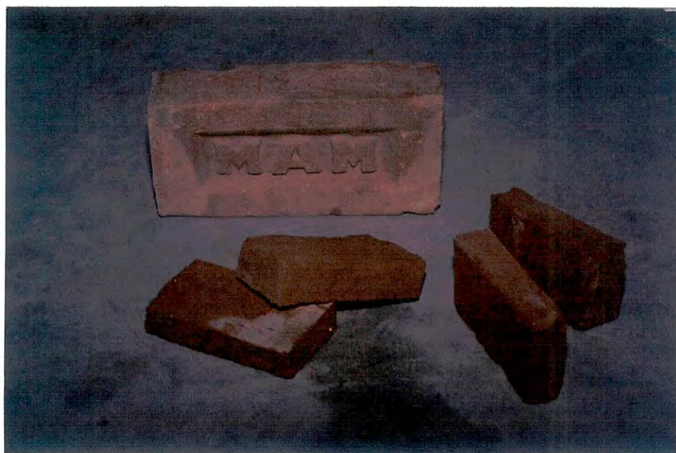
Fig.: 3.12 Samples of half scale masonry brick sliced from full size brick.
