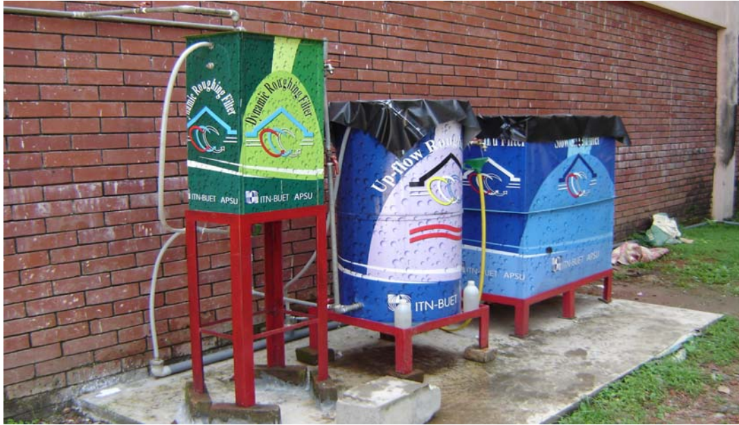
Figure-3.2: Front View of the Laboratory Multistage Filtration Units
