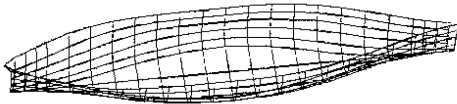
Fig: 4.03 Full body mesh arrangement of Series 60 vessel (Top view)
