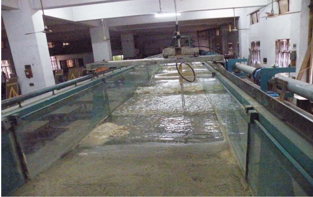
Photograph 4.2.9: Placement of E.M.S at different depth
