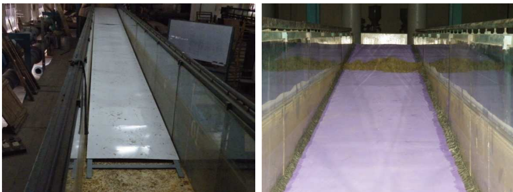
Photograph 4.2.4: Construction stage of artificial slope
