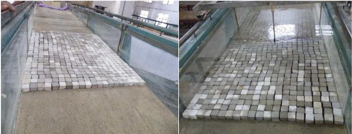
Photograph 4.2.7: Placement of C. C. Blocks
