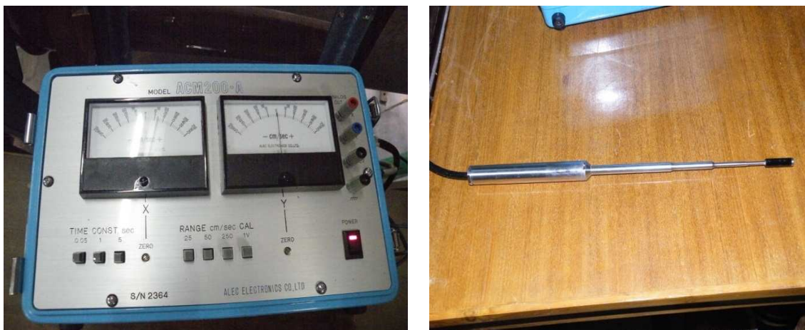
Photograph 4.2.8: Programmable velocity meter (E.M.S)
