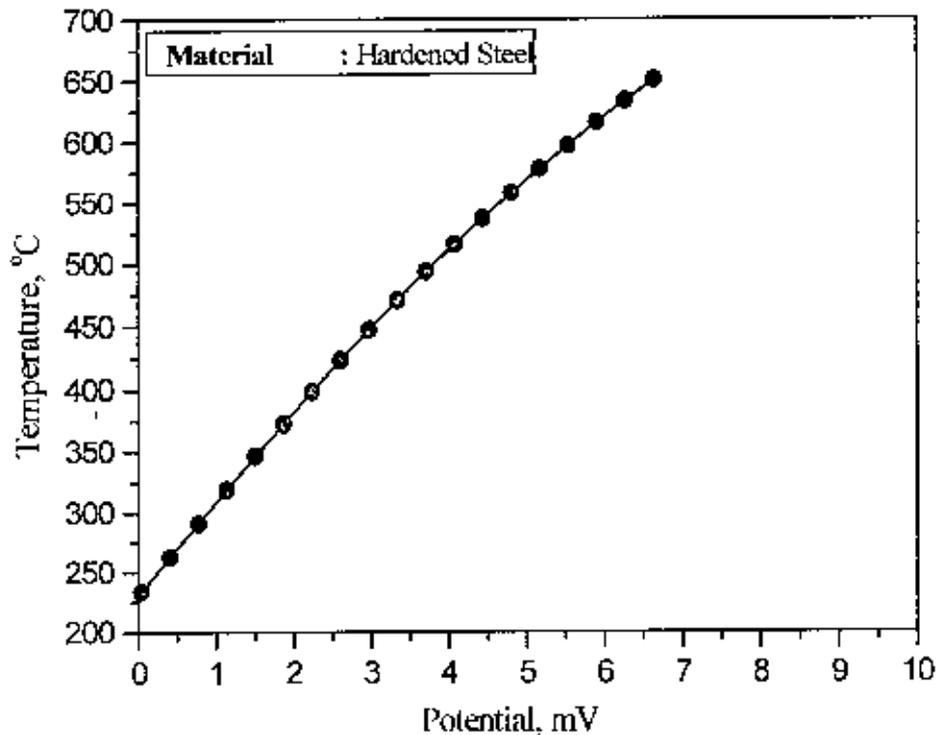
Fig. 4.2 Temperature calibration curve for hardened steel and carbide.
