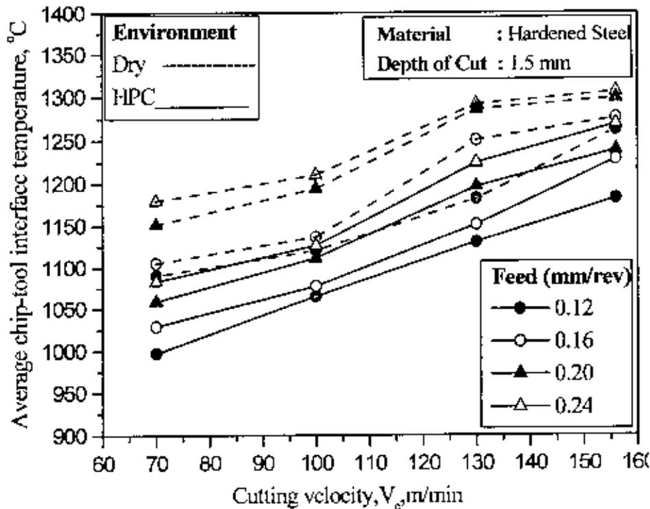
Fig. 4.3 Variation in average chip-tool interface temperature with cutting velocity,  $V_c$  and feed rate,  $S_0$  in turning hardened steel under **dry** and **High-pressure coolant** condition
