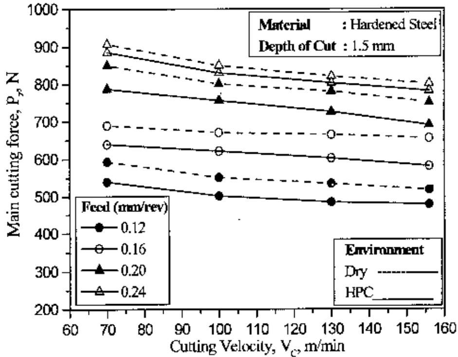
Fig. 4.4 Variation in main cutting force,  $P_z$  with cutting velocity,  $V_c$  and feed rate,  $S_o$  in turning hardened steel under **Dry** and **High-pressure coolant** condition
