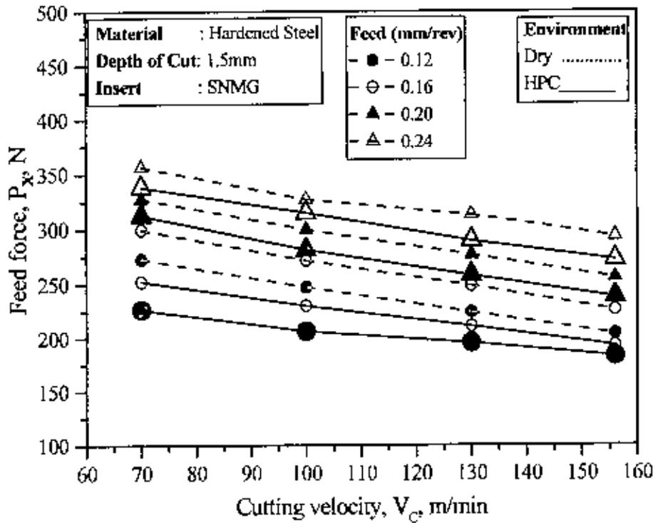
Fig. 4.5 Variation in feed force,  $P_x$  with cutting velocity,  $V_c$  and feed rates,  $S_o$  under Dry and High-pressure coolant condition.
