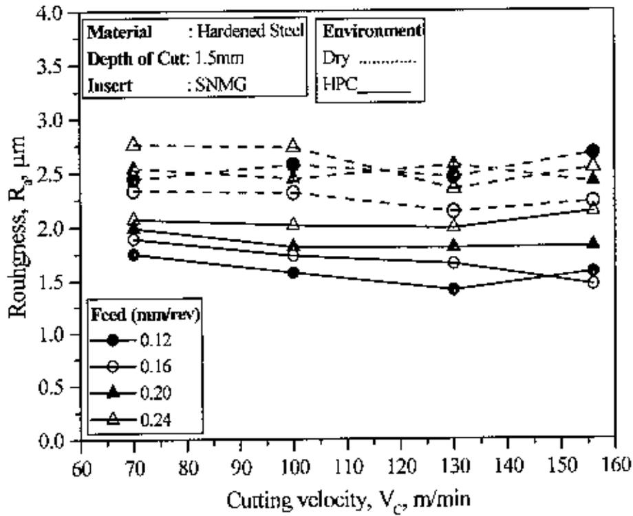
**Fig. 4.6** Variation in surface roughness with cutting velocity,  $V_c$  and feed rates,  $S_o$  under **Dry** and **High-pressure coolant** condition.
