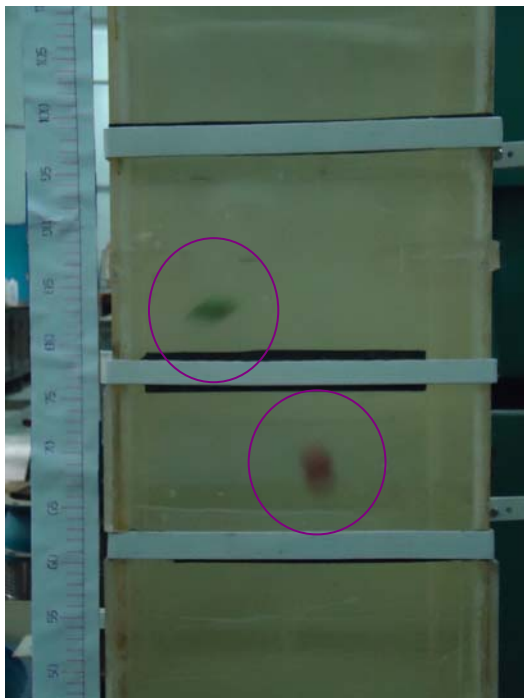
Photograph 4.10(a): Fall velocity measurement
