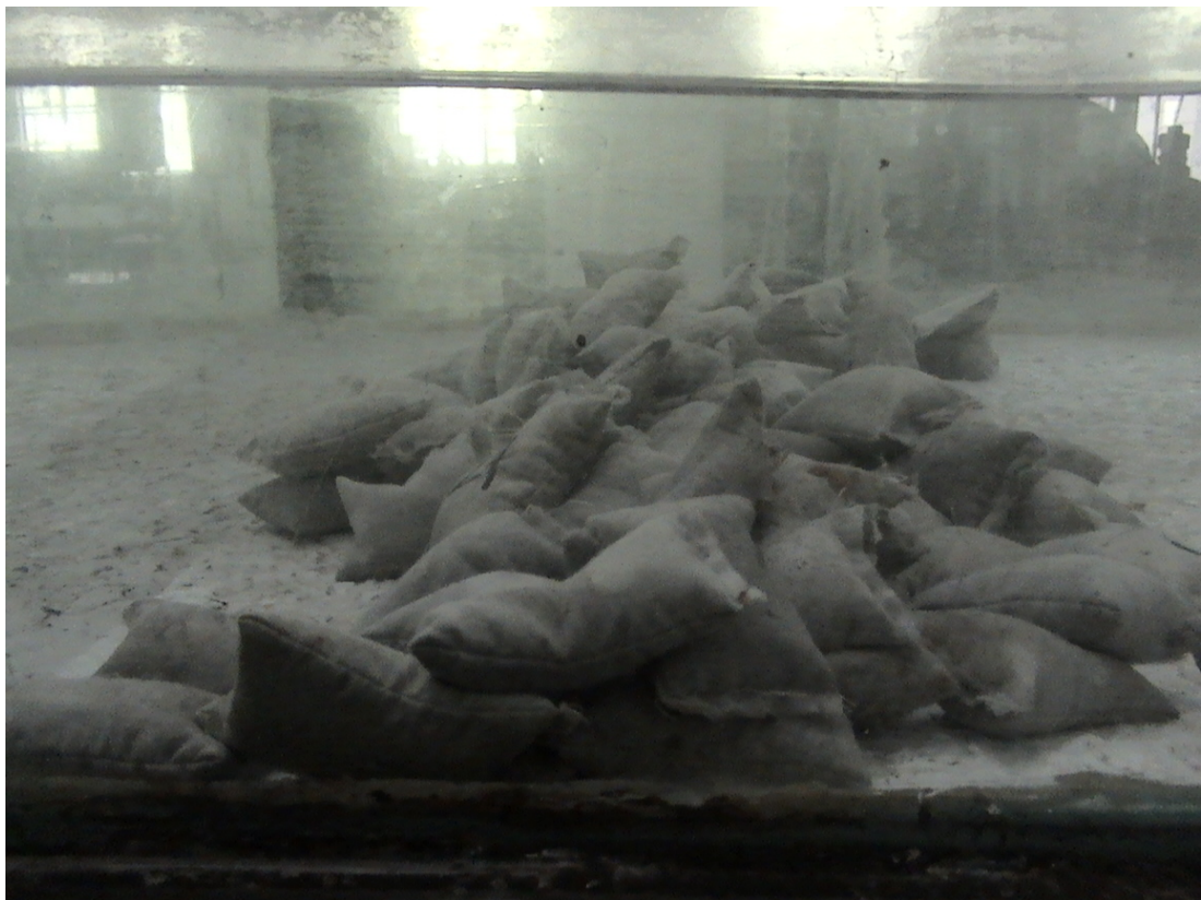
Photograph 4.13: Investigation of threshold condition of geobag
