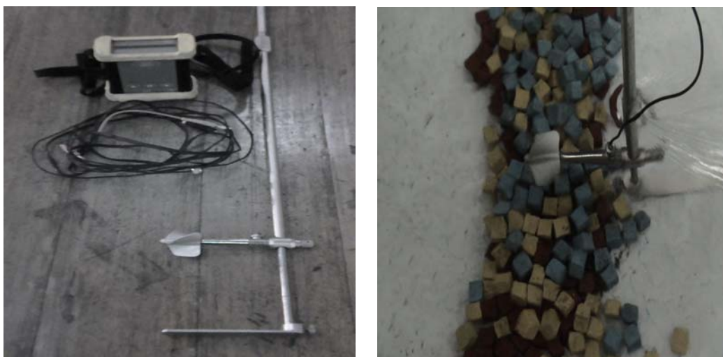
Photograph 4.4(a): Small current meter Photograph 4.4(b): Velocity measurement using current meter
