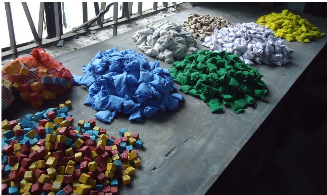
Photograph 4.7: CC blocks and geobags used in experiments
