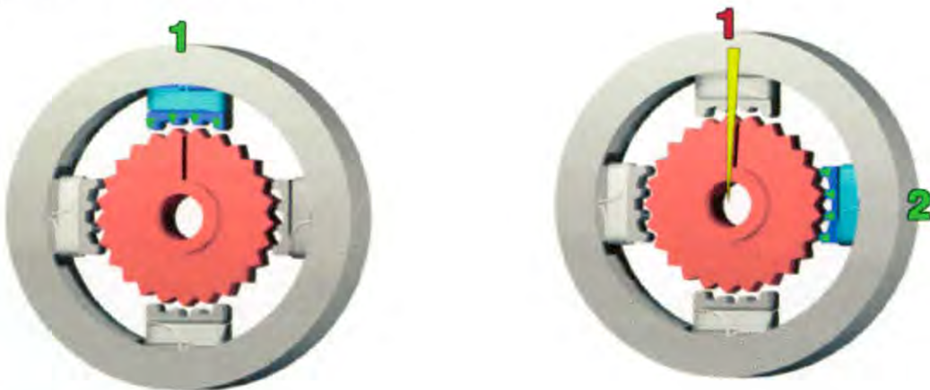
Figure 2.2 Position of the rotor changing as the current supplied to the stator changes [9]
