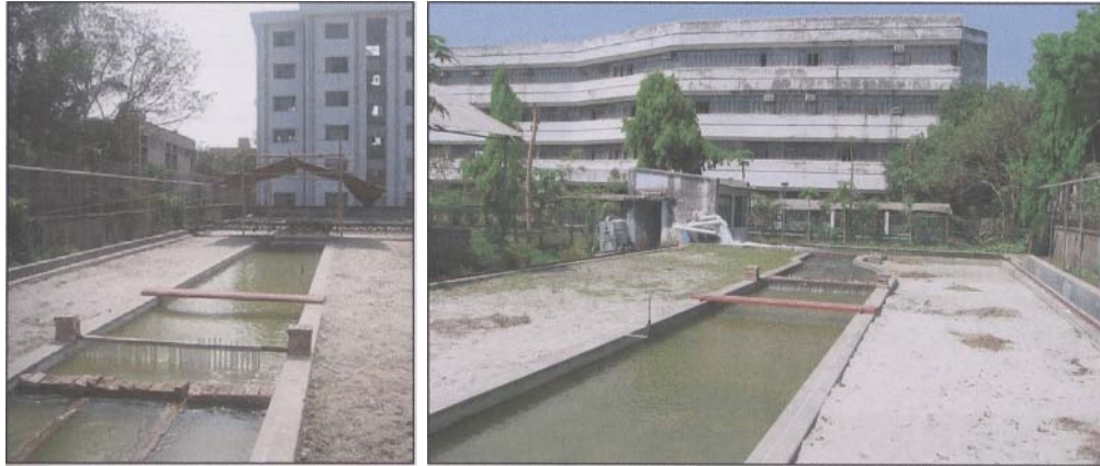
Photograph 4.2: The straight flume with fixed bed in downstream (1) and upstream (r) direction
