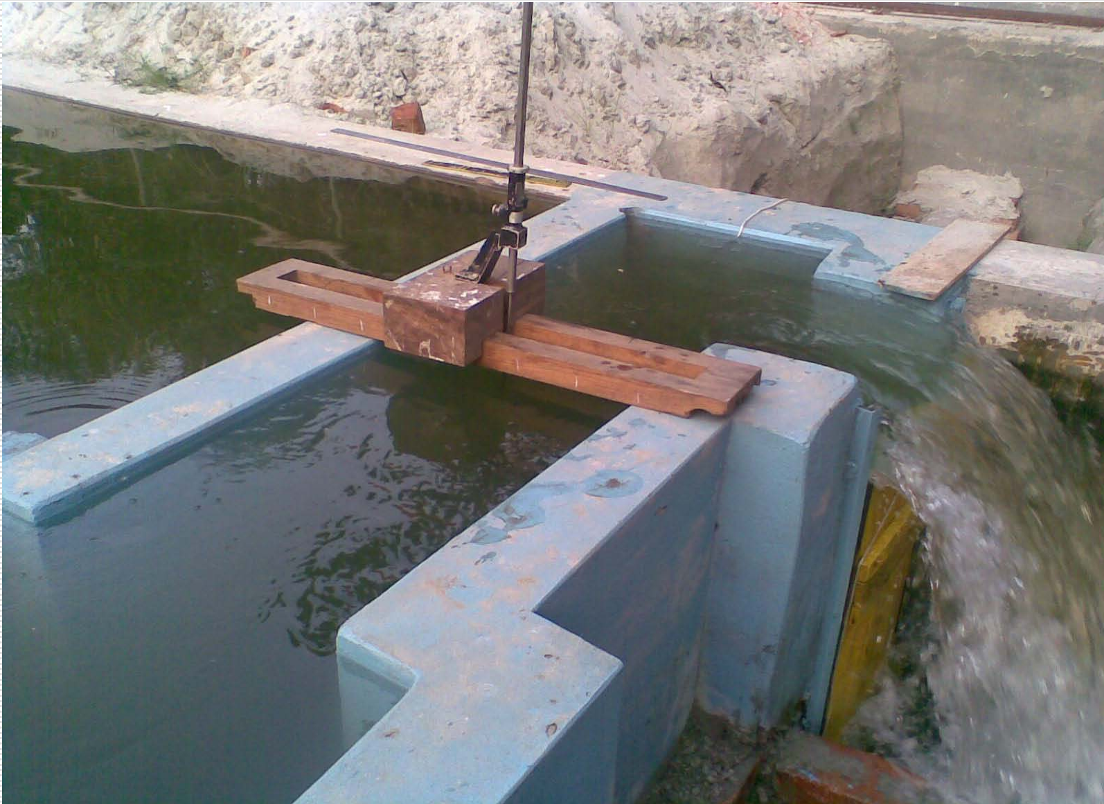
Figure : Model is runs highest gate height and high discharge. (discharge= 0.0927 m 3 /s and gate height=882mm)
