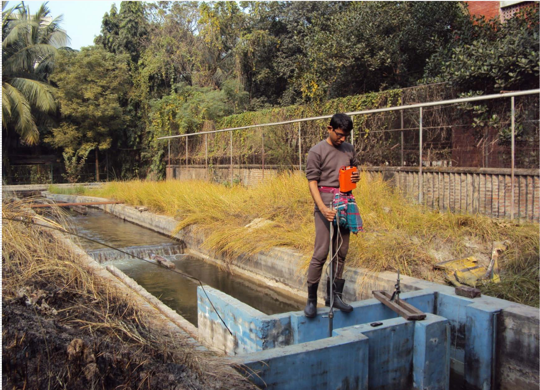
Figure : Measurement of velocity at diversion structure with current meter.
