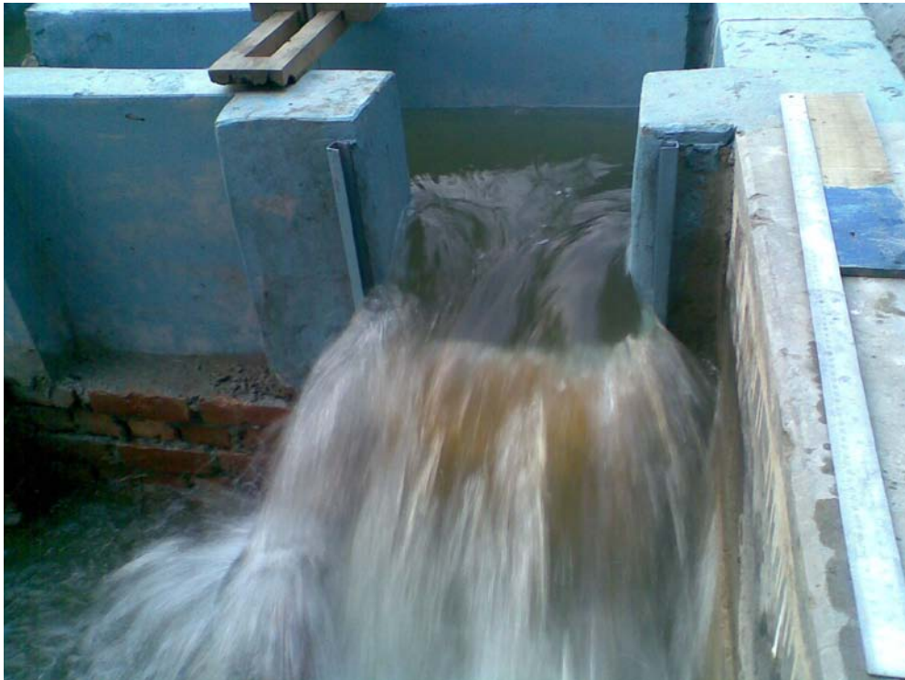
Photograph 4.23: Model is running low gate height and high discharge. (discharge= 0.0928 \text{ m}^3/\text{s} and gate height= 201 \text{ mm} )
