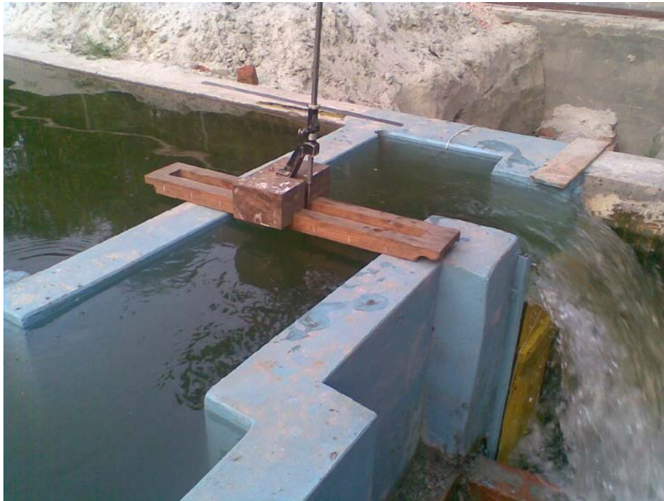
Photograph 4.27: Model is runs highest gate height and high discharge. (discharge= 0.0927 \text{ m}^3/\text{s} and gate height=882mm)
