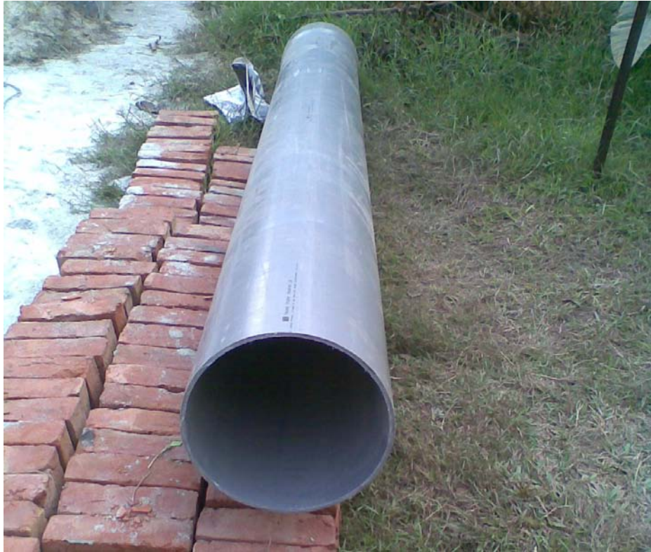
Photograph 4.14: 12" dia diversion pipe
