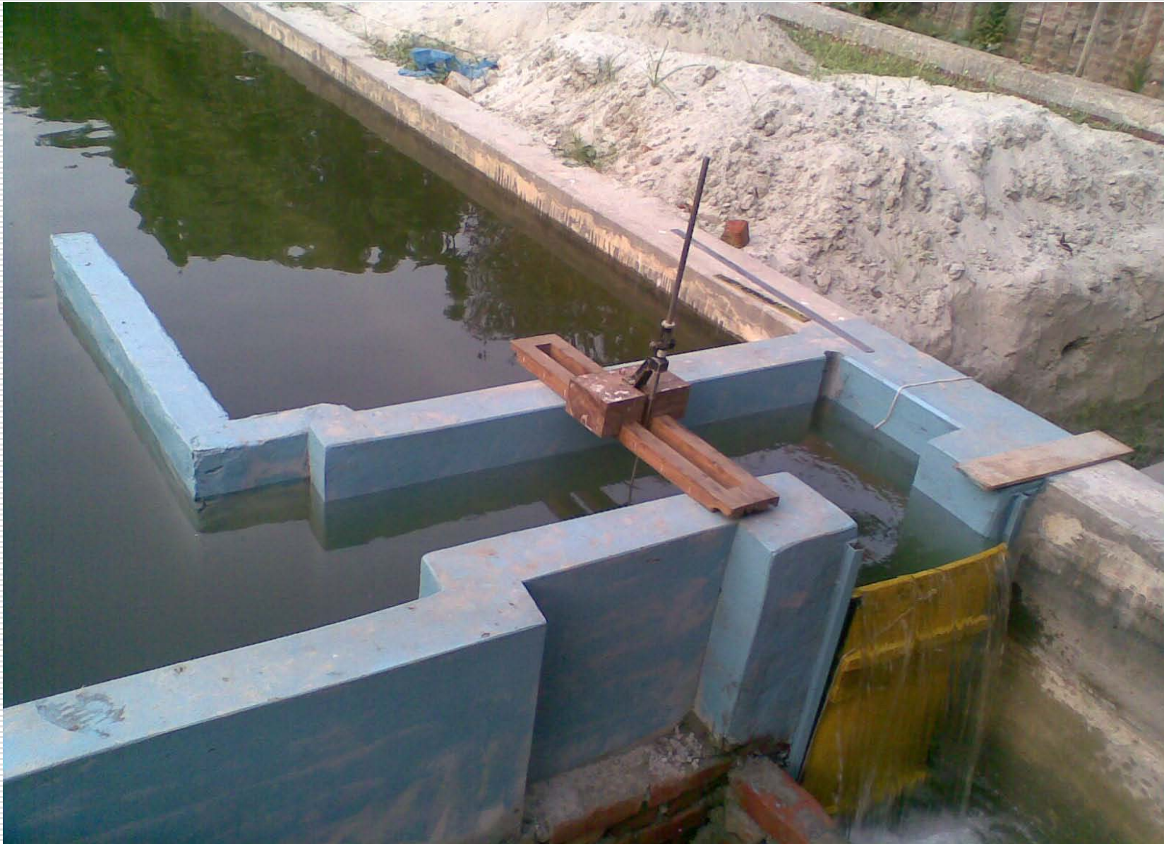
Figure : Eight run of the model (discharge= 0.0574 \text{ m}^3/\text{s} and gate height=736mm)
