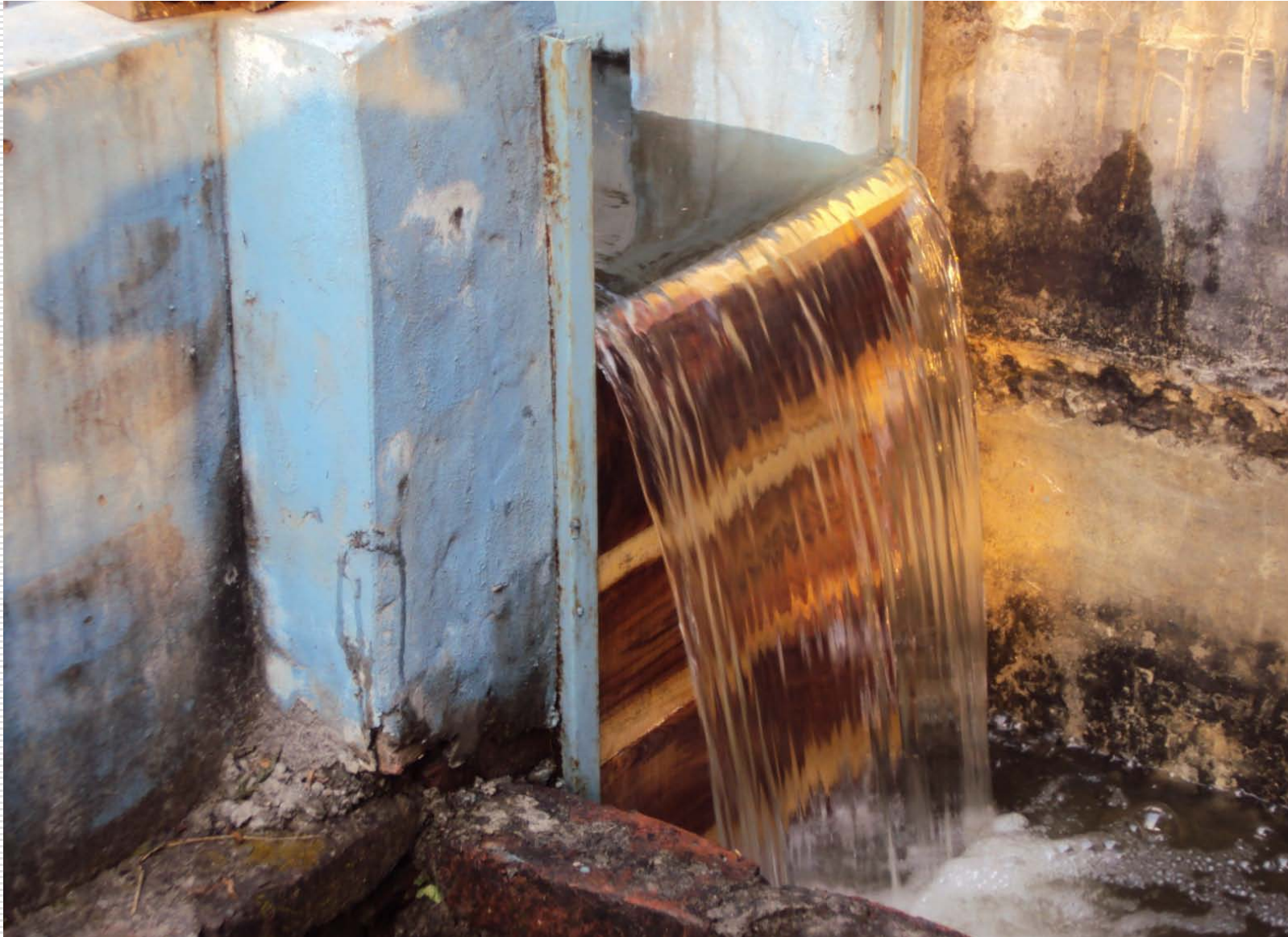
Figure : Model is running average gate height and low discharge (discharge= 0.0443 \text{ m}^3/\text{s} and gate height=484mm)
