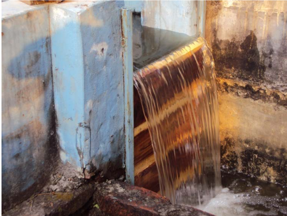
Photograph 4.24: Model is running average gate height and low discharge (discharge= 0.0443 \text{ m}^3/\text{s} and gate height=484mm)
