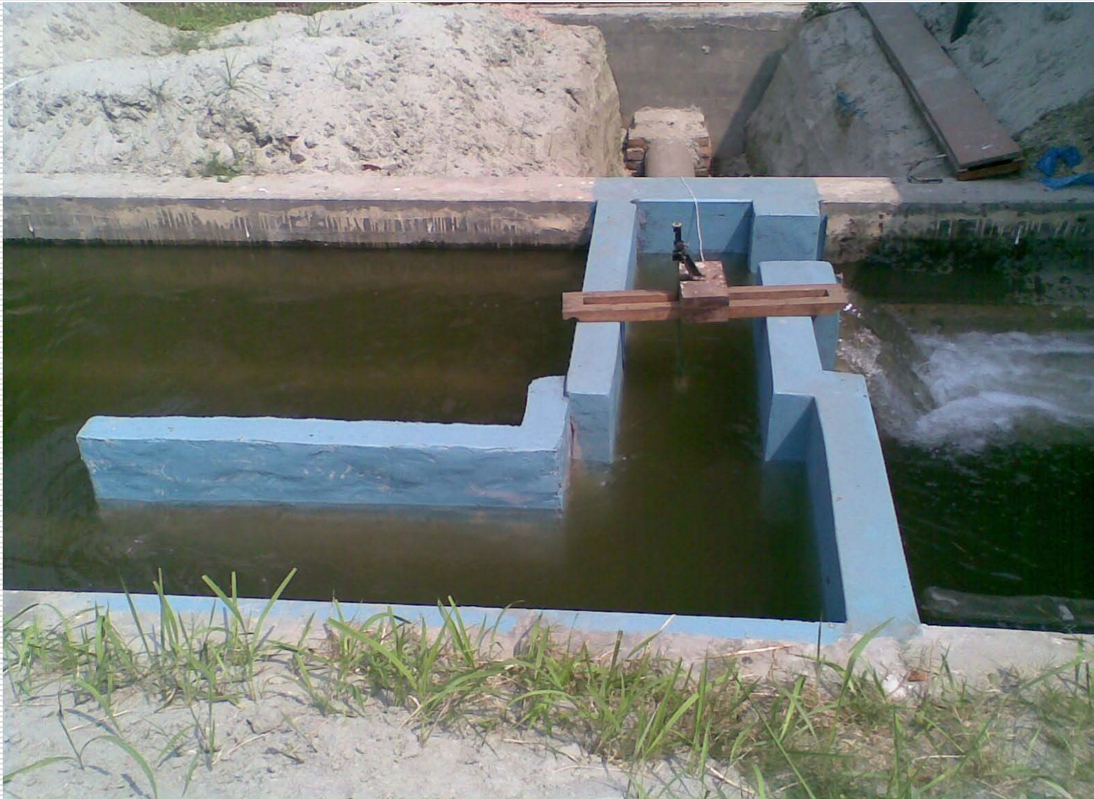
Figure : Model is running on it's average capacity (discharge= 0.0901 m 3 /s and gate height=412mm)
