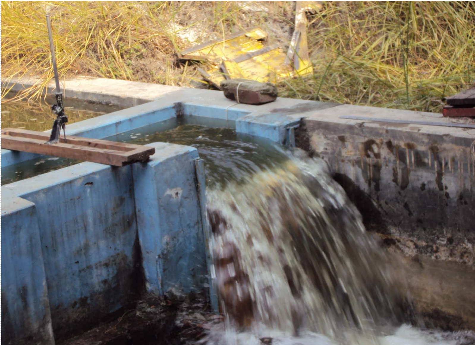
Figure : Model is running highest gate height and high discharge. (discharge= 0.109 \text{ m}^3/\text{s} and gate height=692mm)
