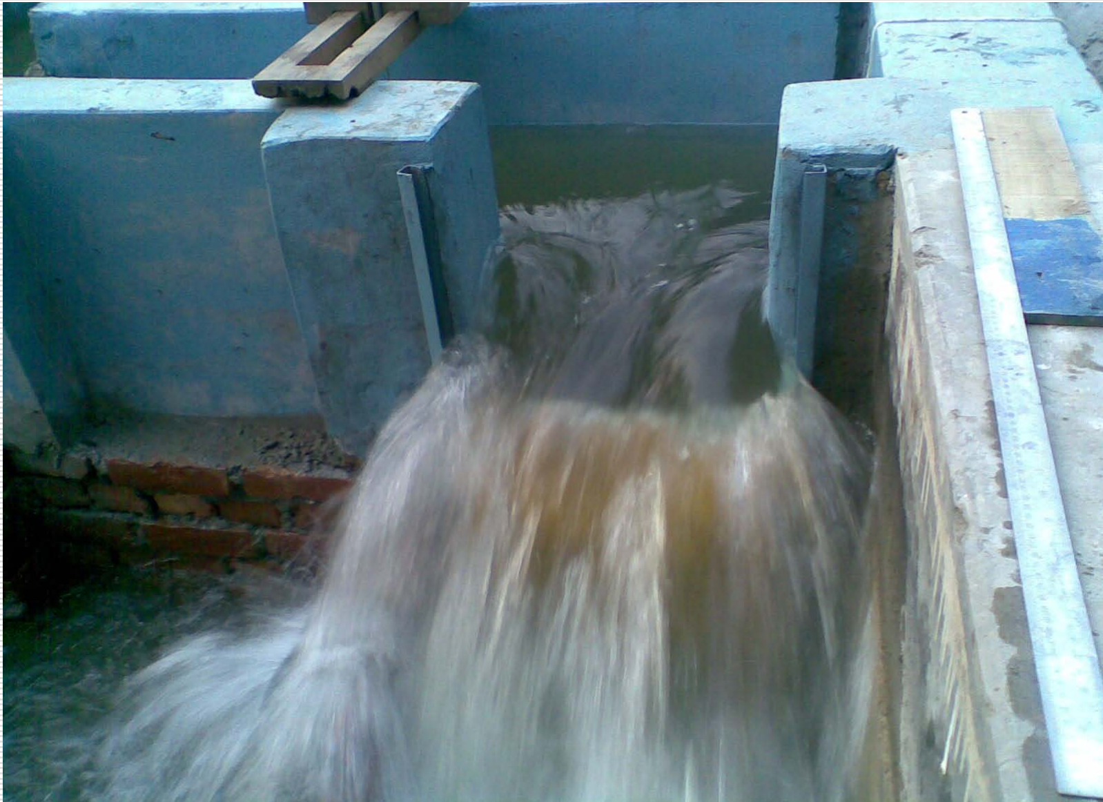
Figure : Model is running low gate height and high discharge. (discharge= 0.0928 \text{ m}^3/\text{s} and gate height=201mm)
