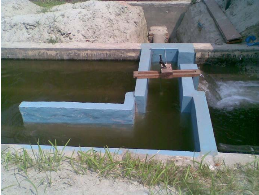
Photograph 4.26: Model is running on it's average capacity (discharge= 0.0901 \text{ m}^3/\text{s} and gate height=412mm)
