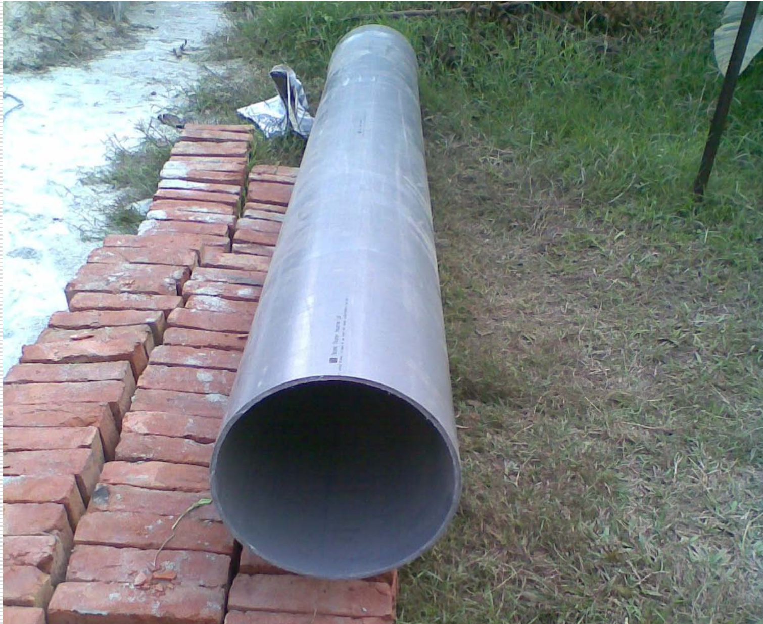
Figure : 12”dia diversion pipe
