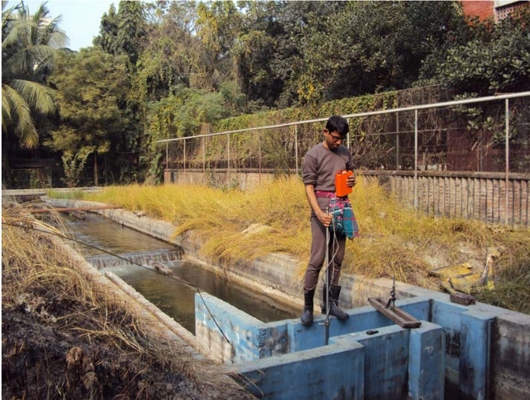
Photograph 4.22: Measurement of velocity at diversion structure with current meter.
