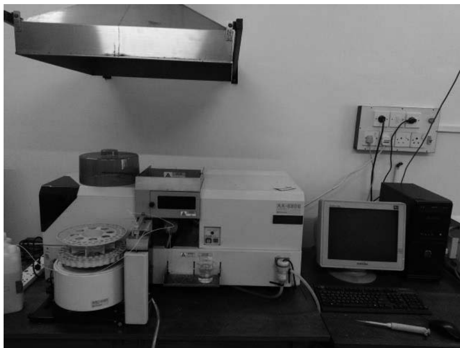
Figure 3.36: Machine for \text{Ca}^{2+} Ions Determination by Atomic Absorption Method
