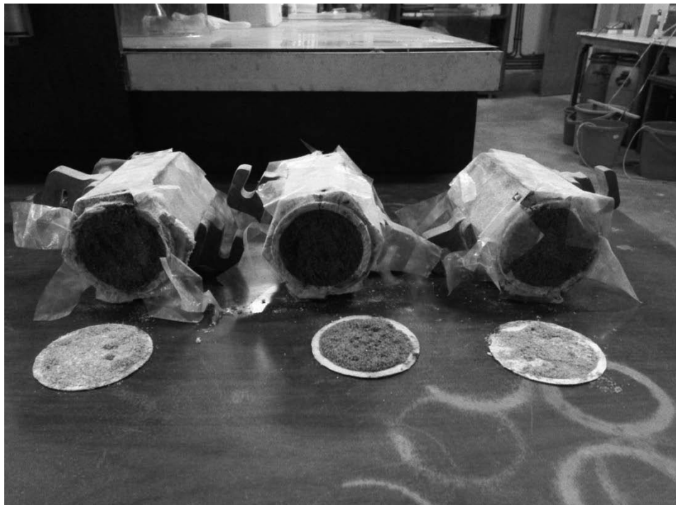
Figure 4.6: Presence of Precipitated \text{CaCO}_3 at the Bottom of the Specimens in Method A
