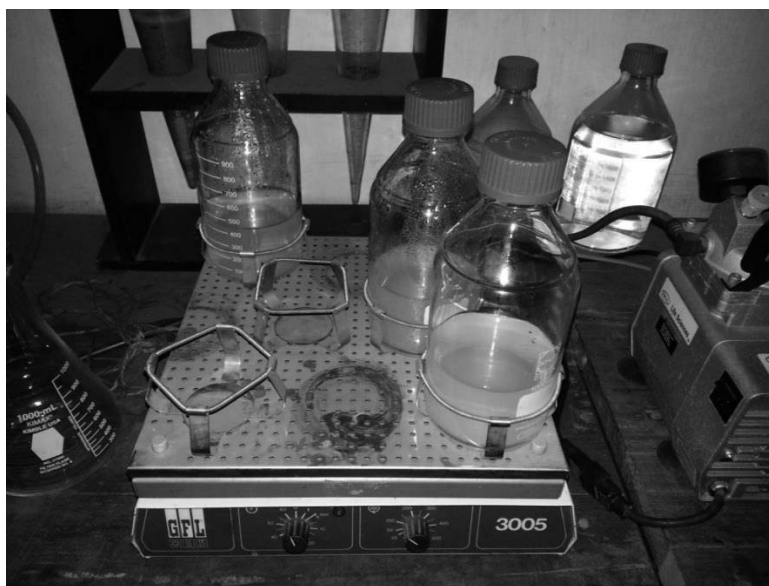
Figure 3.34: Urea Nutrient Solution with NH 4 -YE Medium and Bacteria at Room Temperature over a Shaker
