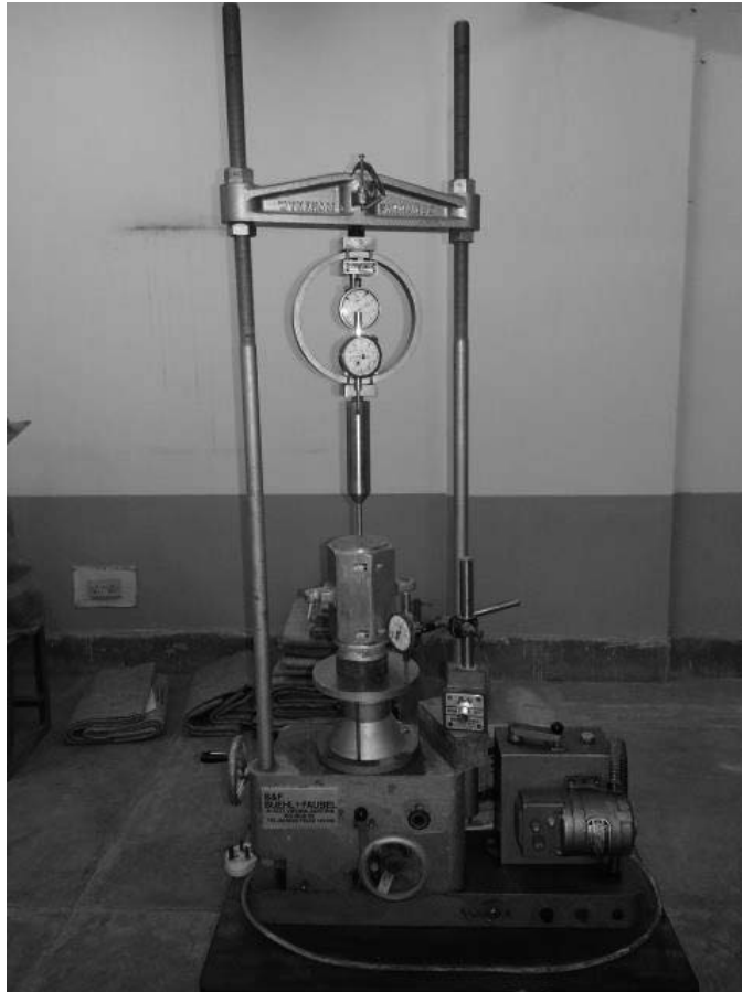
Figure 3.37: Compression Machine for Needle Penetration Test
