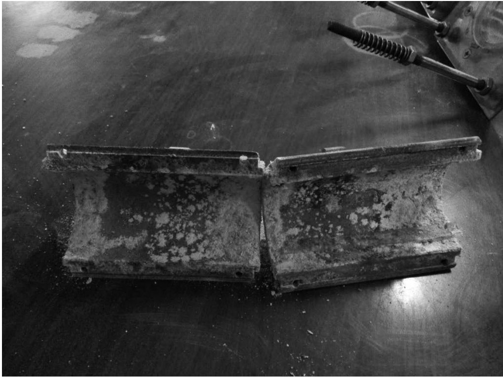
(a) \text{CaCO}_3 at the Inside Wall of the Mold in Method A
