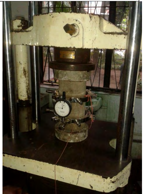
Fig 3.20: Measurement of Stress-strain
