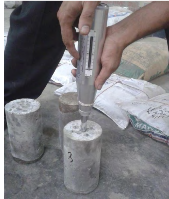
Fig 5.2: RH (Schmidt hammer) testing method
