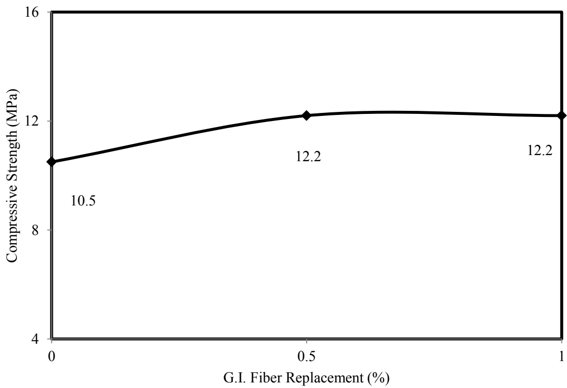
Fig 5.6: Compressive strength(NDT) of RB concrete at 7 day
