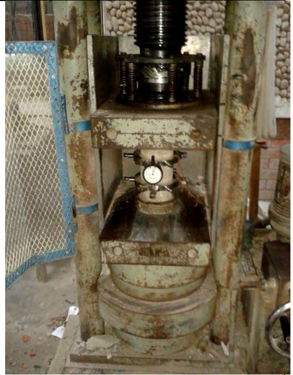
Fig 3.18: Compressive strength test
