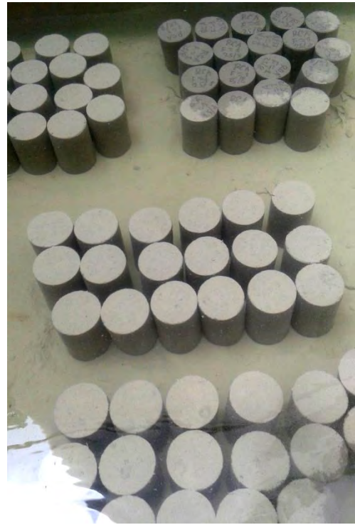
Fig 3.16: Under water curing of specimens
