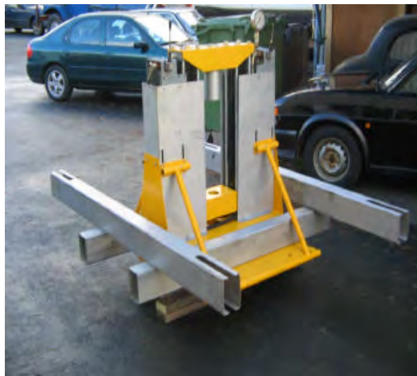
Figure C4 Long beams on top of the short ones
