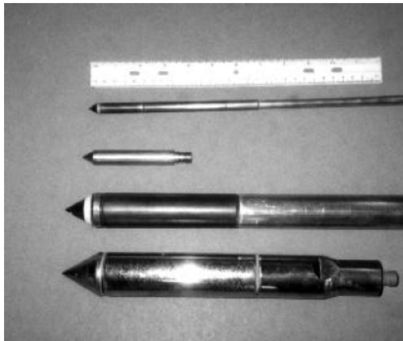
(a) Schematic of the electric friction cone penetrometer
