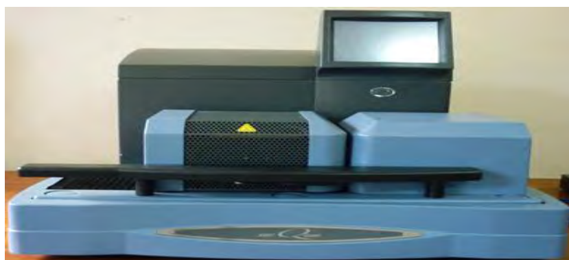
Fig.3.14: DSC & TGA analyzer (TA instrument, SDT Q-600)
