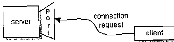
Fig. 4.1: Connection request from client to a server port.
