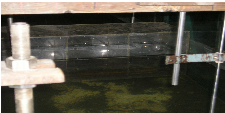
Photograph A7: Breakwater in floating condition
