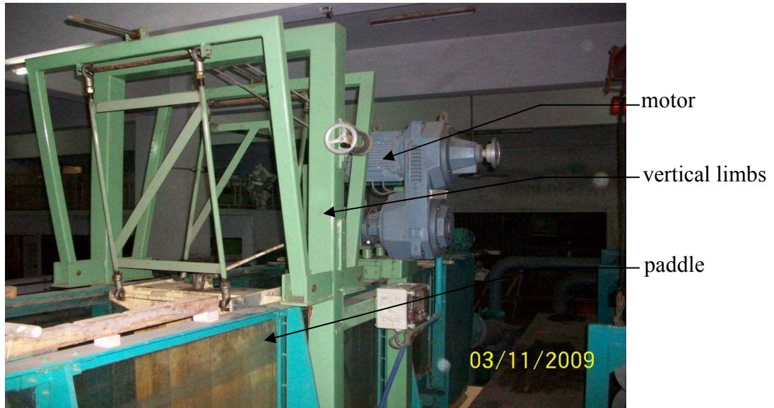
Photograph 3.4.4: Wave generator labeling with main parts
