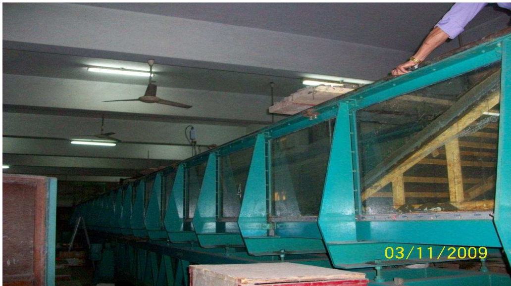
Photograph 3.4.3: Laboratory flume with bank slope
