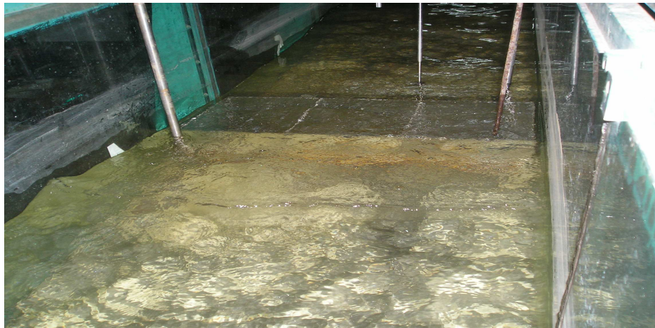
Photograph A6: Breakwater in submerged condition
