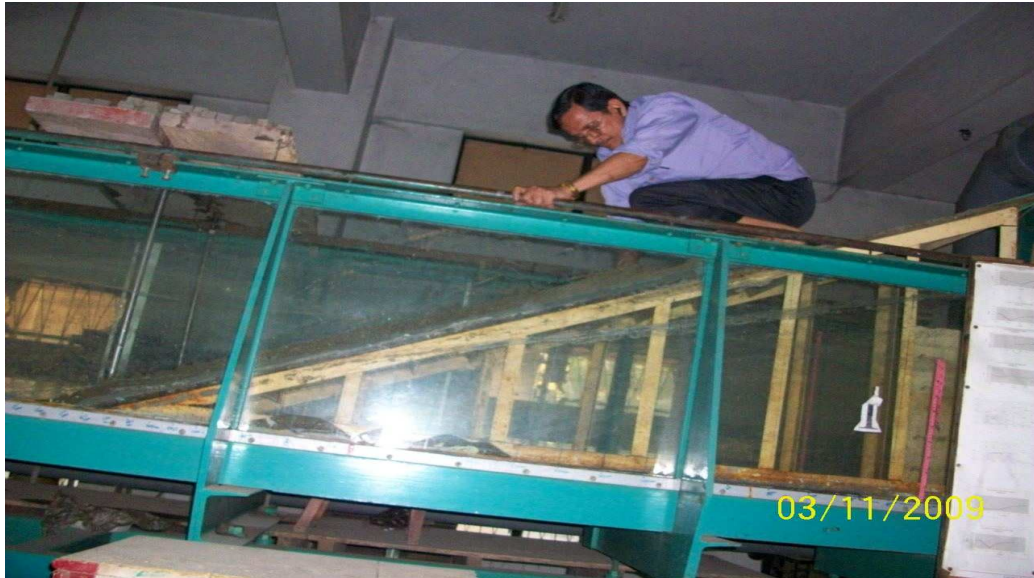
Photograph 3.4.7: Preparing a bank slope
