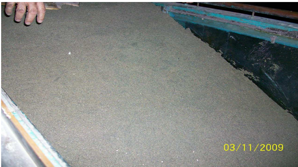
Photograph 3.4.8: Sand layer over the acrylic plate
