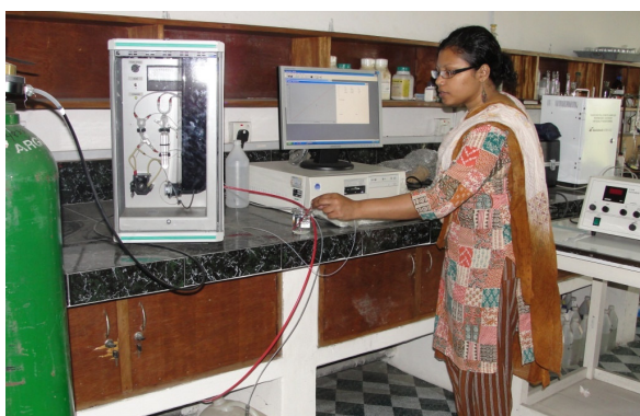
Photo 3.2 TOC Analysis in Environmental Science Discipline Laboratory, KU
