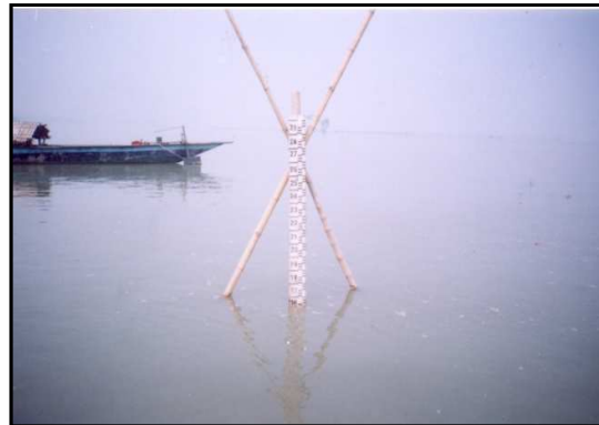
Figure 3.6: Water level gauge on the River Jamuna
