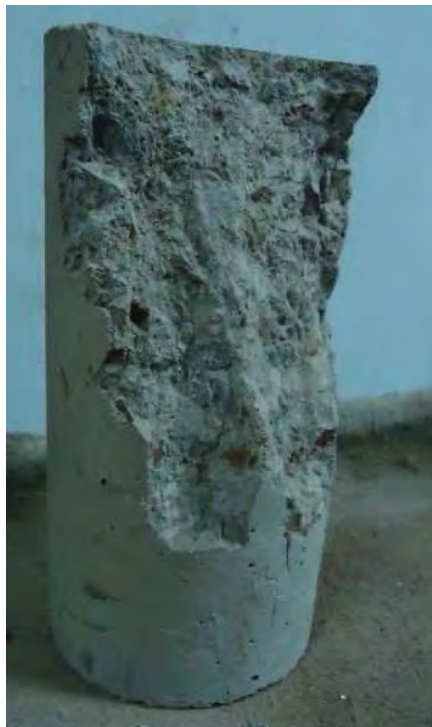
Figure C.16 Failure pattern after testing
