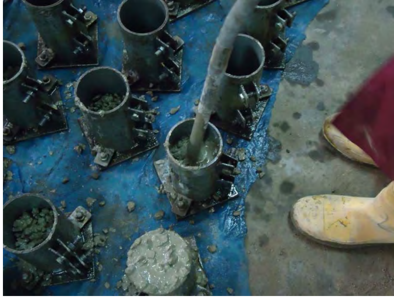
Figure C.9 Compaction of concrete sample
