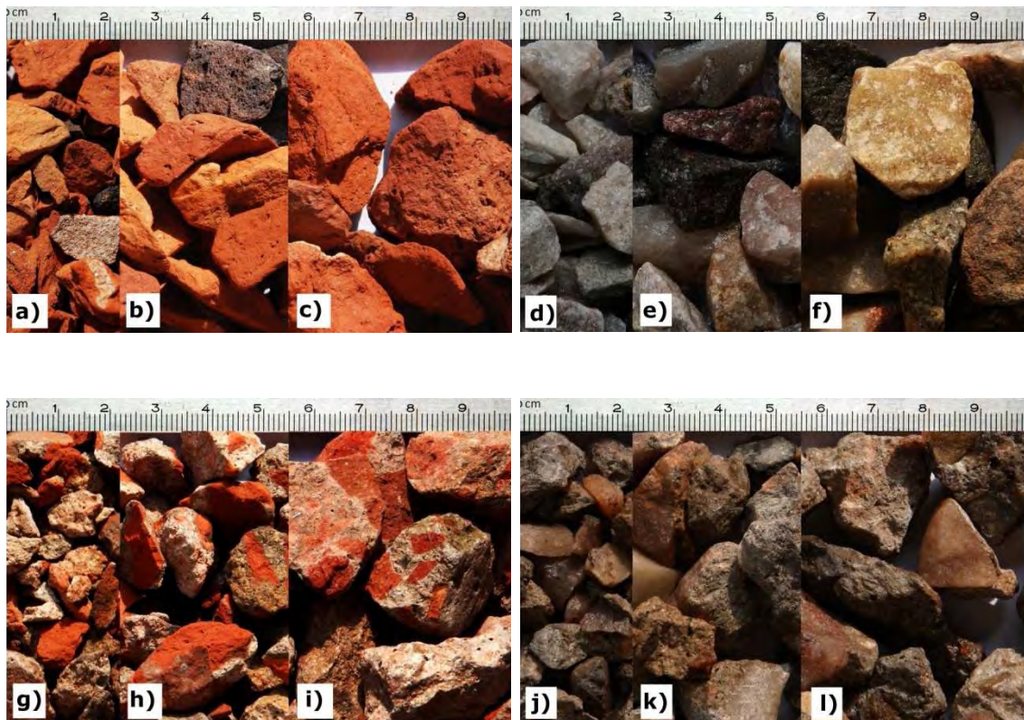
Figure 3.1 Types of coarse aggregate used in the research (a), (b), (c) are brick aggregates, (d), (e), (f) are stone aggregates, (g), (h), (i) are recycled brick aggregates and (j), (k), (l) are recycled stone aggregates. Here (a), (d), (g), (j) are 6.5mm passing and 4.75mm retained, (b), (e), (h), (k) are 12.5mm passing and 6.5mm retained and (c), (f), (i), (l) are 19mm passing and 12.5mm retained.
