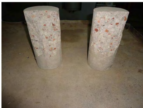
Figure 4.2 Concrete specimens after burning and testing
