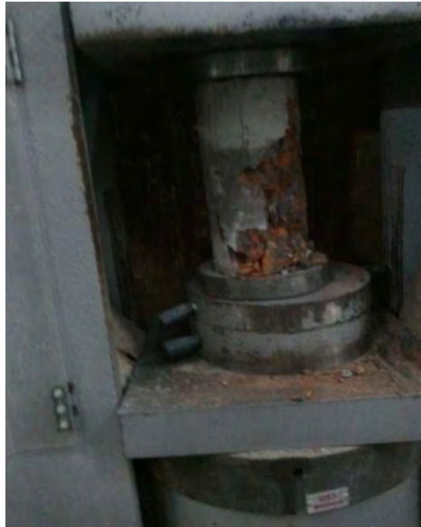
Figure C.15 Crushing strength test
