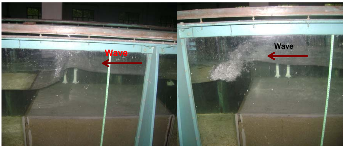
Fig. 2.6 (d): Wave breaking at the onshore end of the breakwater
