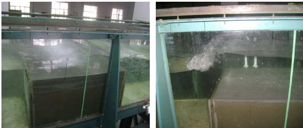
Fig. 2.14 (iii): Collapsing type wave breaking
