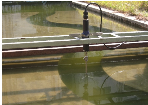
Figure 3.15: Measuring line on the side wall and measuring bridge across the channel
