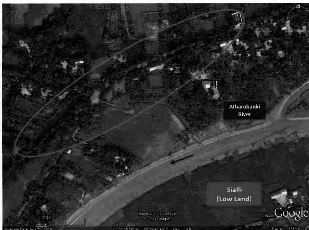
Figure 4-49: Vulnerable area of Z7041 (due to low height embankment) at Sialli
