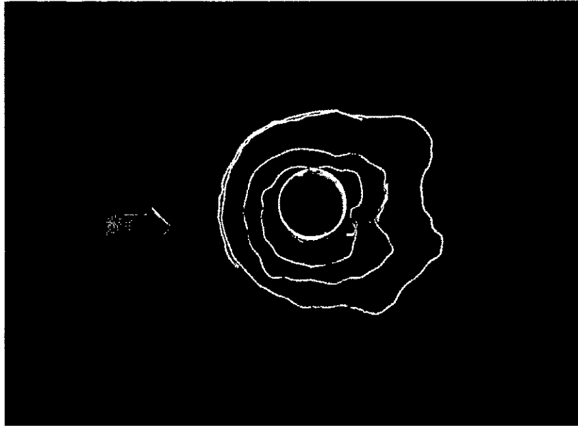
Photograph B.25: Run 13-Bed material 2 ( d_{50} = 0.18 mm)-Circular pier ( l/b=1 )- Q=200 l/s Floodplain
