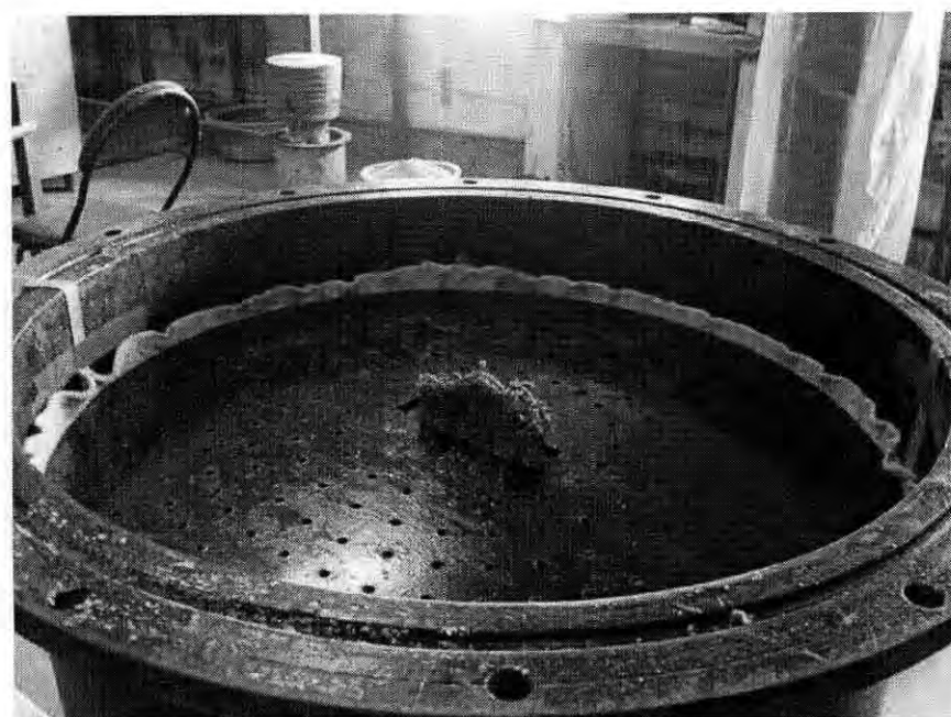
Figure 3.35: Perforated Steel Plate on Top of Geotextile Layer (Test with Jute PVD).
