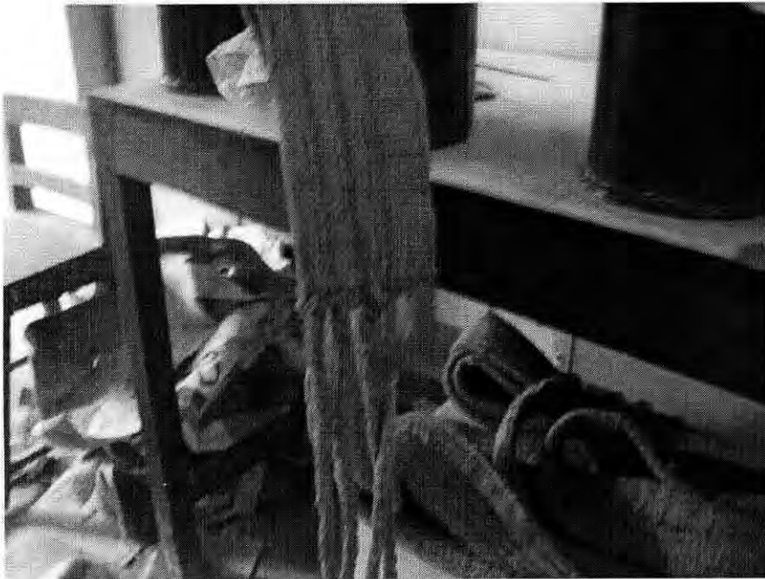
Figure 3.5: Photograph Showing Jute PVD with Jute Rope Core
