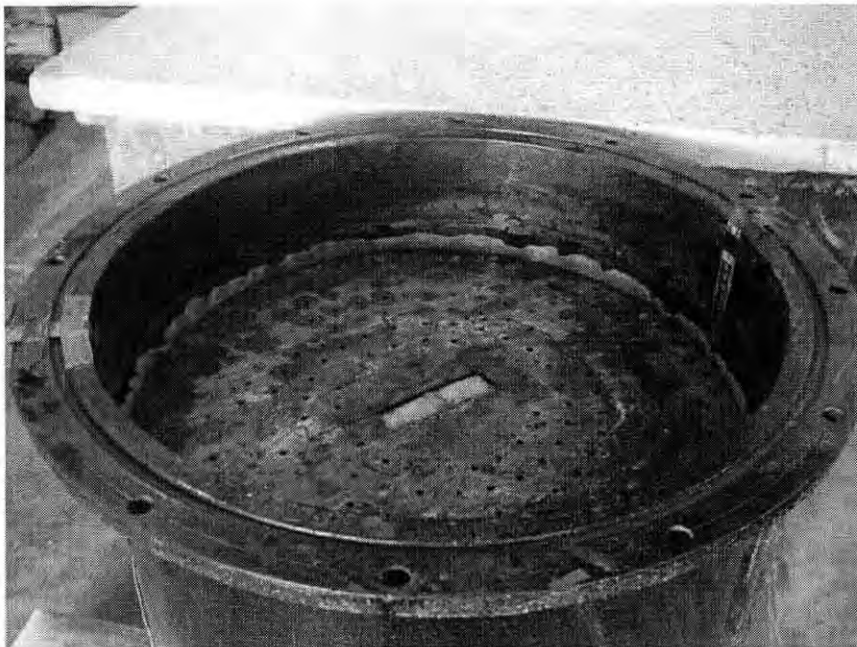
Figure 3.25: Surcharge Removed after 28 Days (Test without Vertical Drains)
