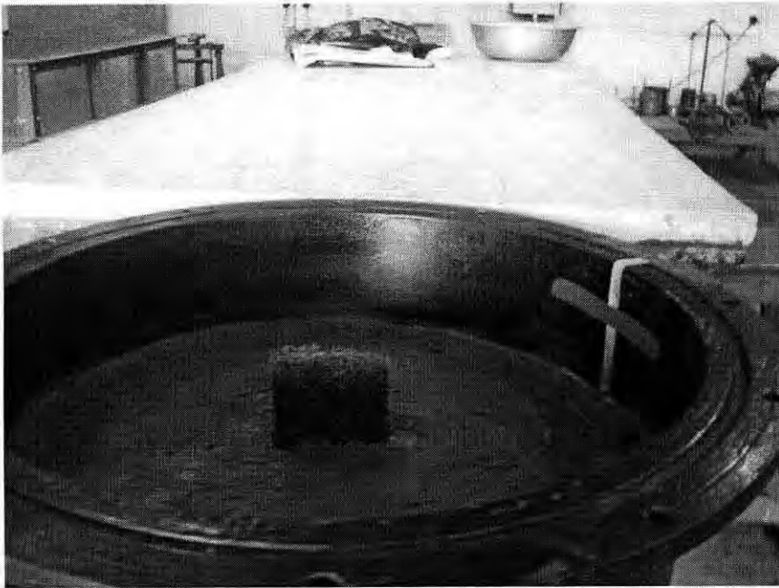
Figure 3.32: Steel Tank Filled with Soil Slurry (Test with Jute PVD).
