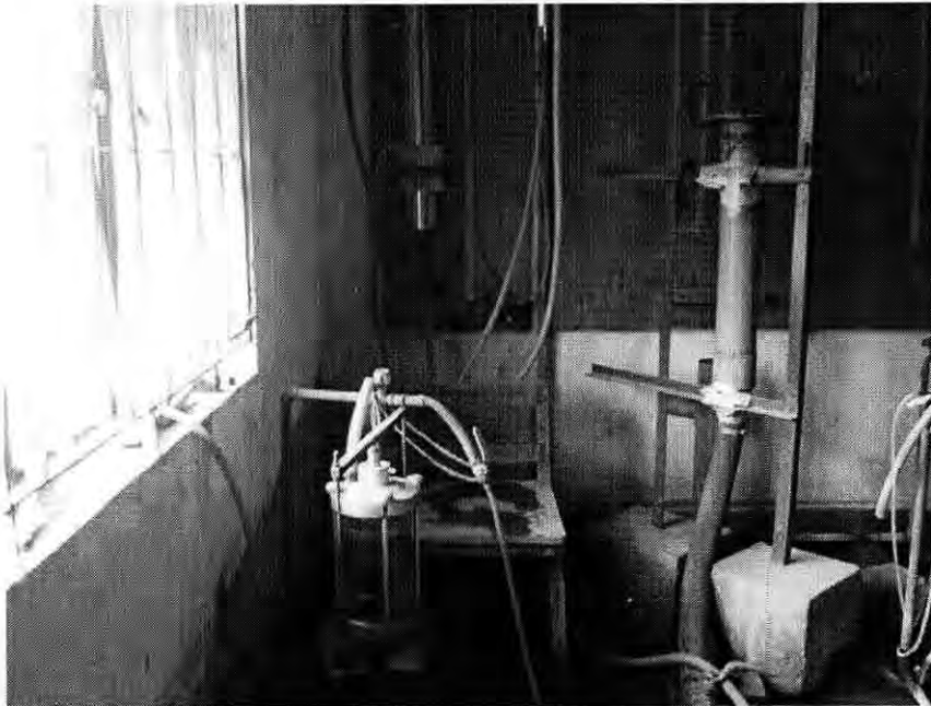
Figure 3.9: Permittivity Test Set-Up Arrangements
