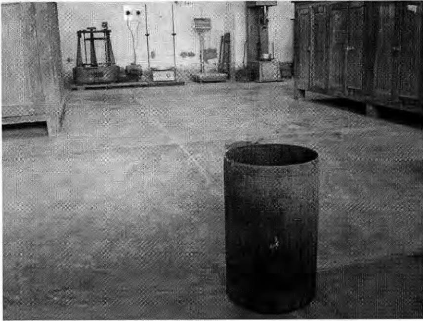
Figure 3.6: Cylinder for Measuring Field Unit Weight.
