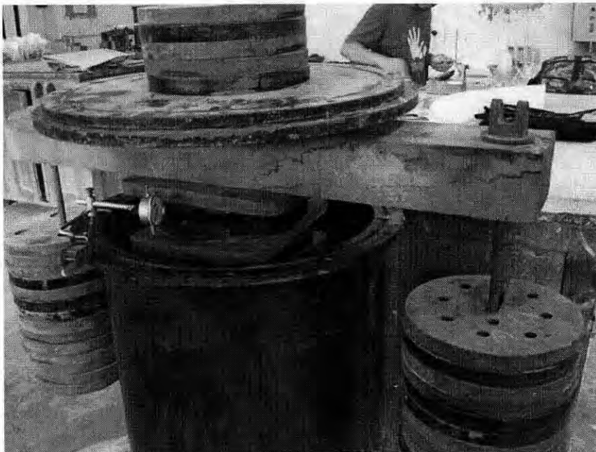
Figure 3.31: Surcharge Load Applied for Soil Settlement (Test with Synthetic PVD).
