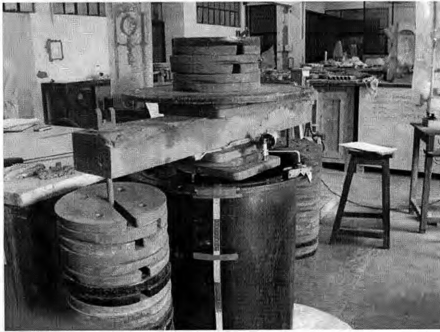
Figure 3.36: Surcharge Load Applied for Settlement (Test with Jute PVD).
