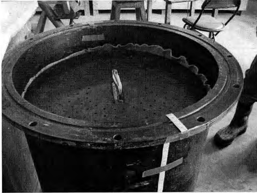
Figure 3.30: Perforated Steel Plate on Top of Geotextile Layer (Test with Synthetic PVD)
