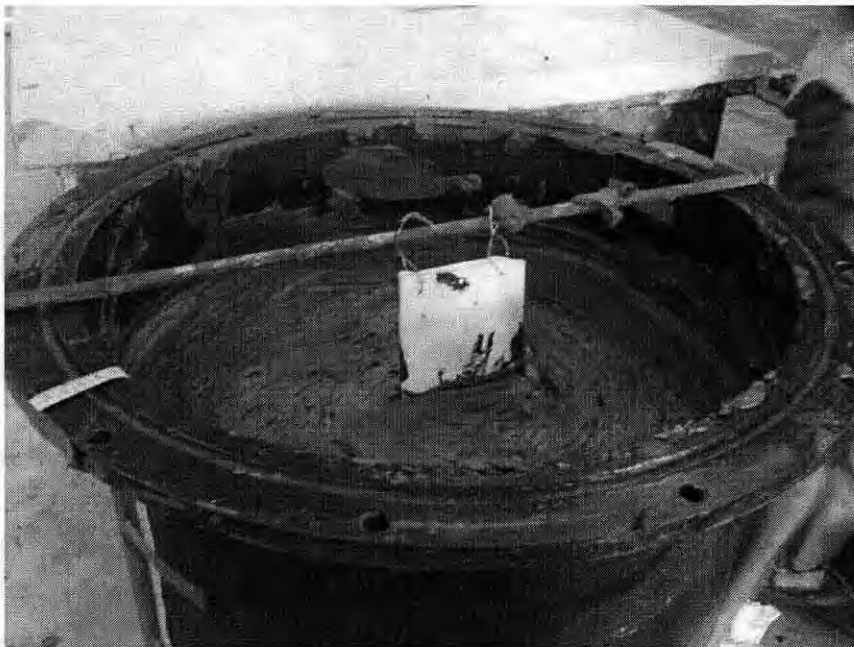
Figure 3.27: Steel Tank Filled with Slurry (Test with Synthetic PVD).
