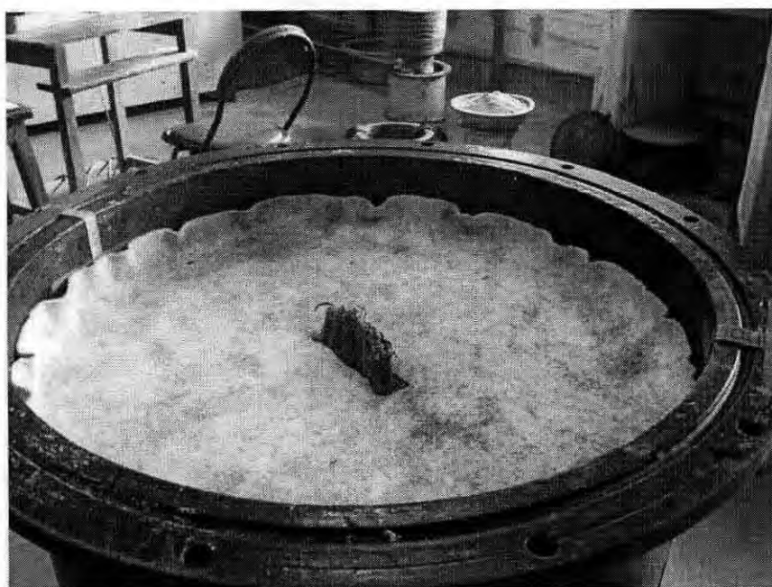
Figure 3.34: Geotextile Filter on Top of Sand Blanket (Test with Jute PVD).
