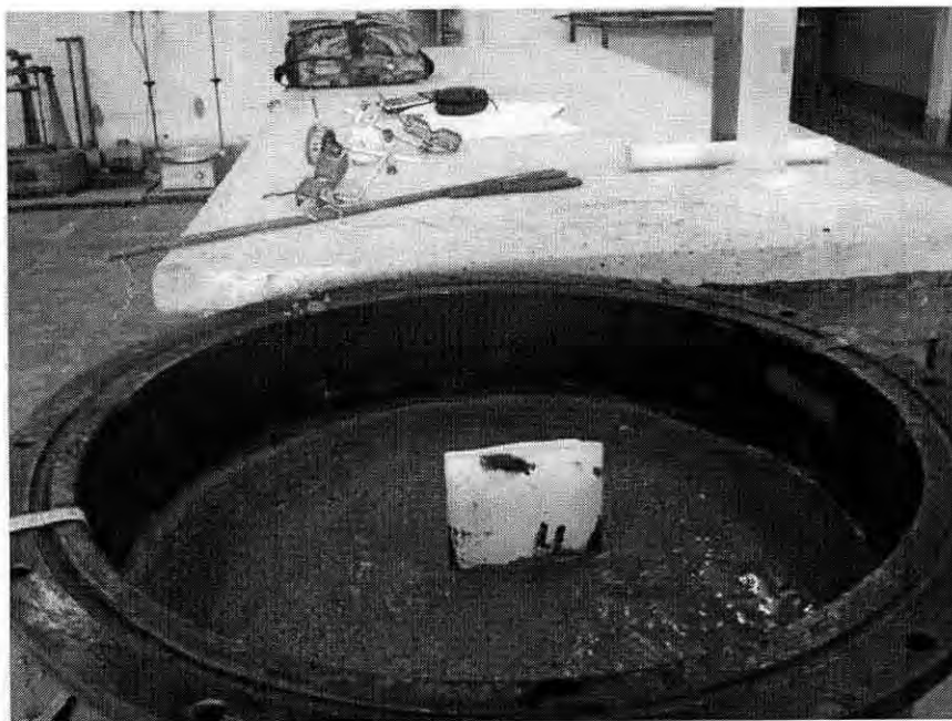
Figure 3.28: Moist Sand Blanket on Top of Slurry (Test with Synthetic PVD).
