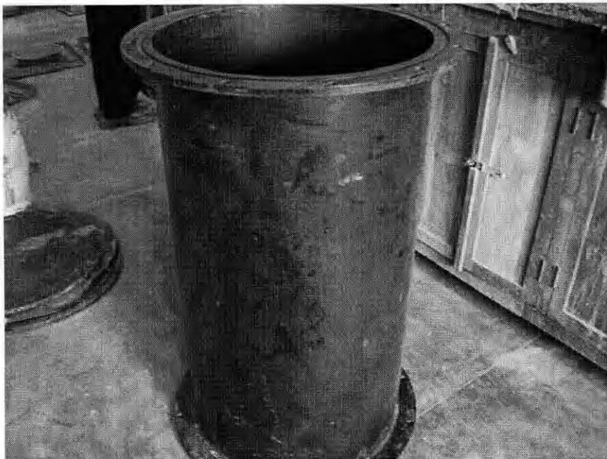
Figure 3.15: Photograph Showing a Steel Tank for Soil Settlement
