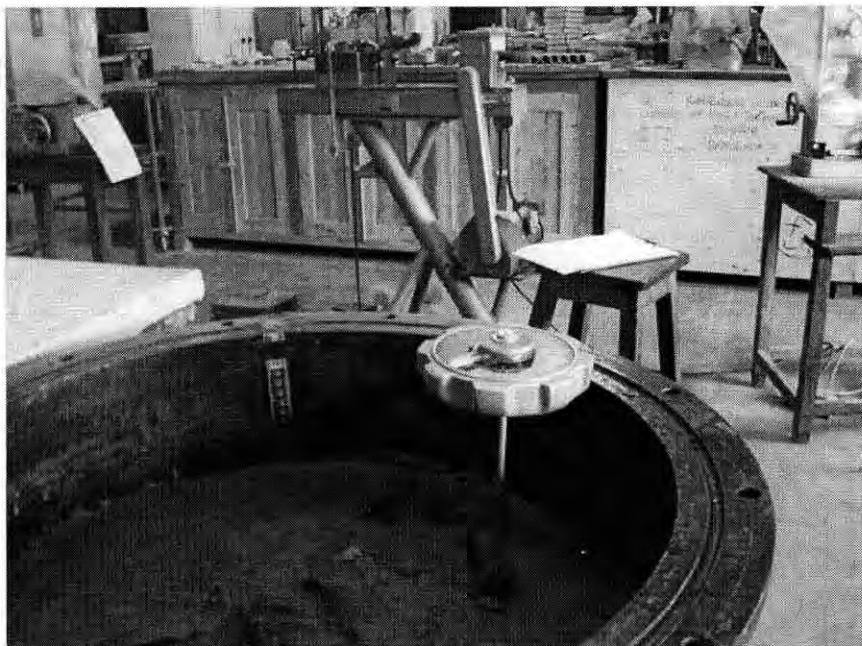
Figure 3.23: Shear Strength Being Measured by Pilcon Hand Vane Tester.
