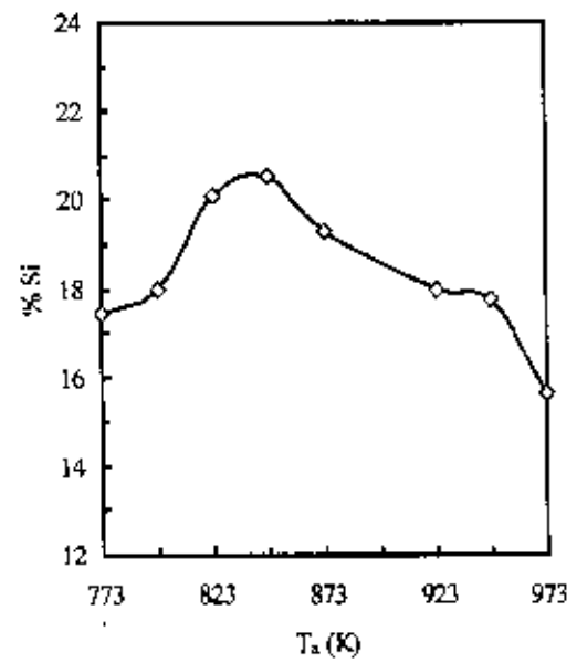
Fig. 4.2.6. Variation of silicon content with annealing temperature, T_a .
