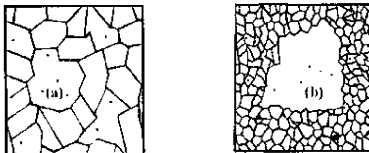
Figure 2.14. Grain growth (a) discontinuous, (b) duplex (schematic) [2].
