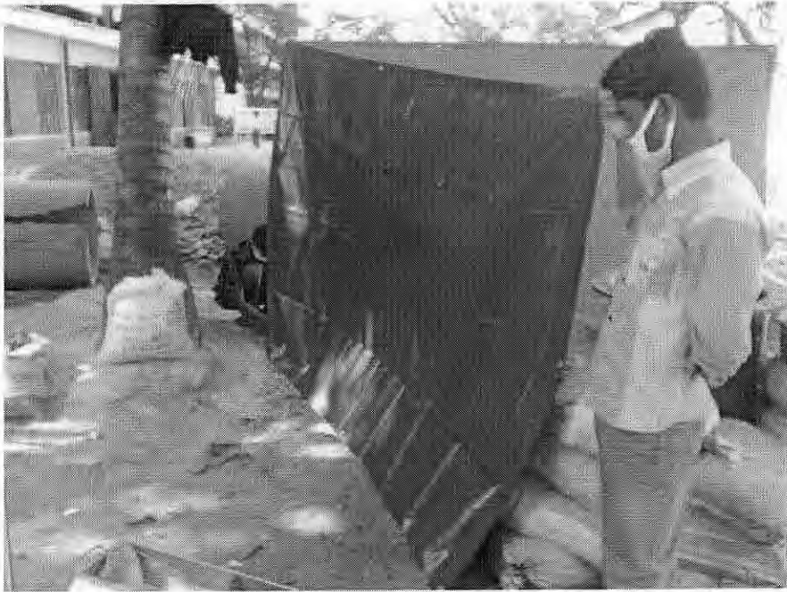
Fig. 3.7: Calibration chamber surrounded by thick polythene sheet to minimize disturbance by wind
