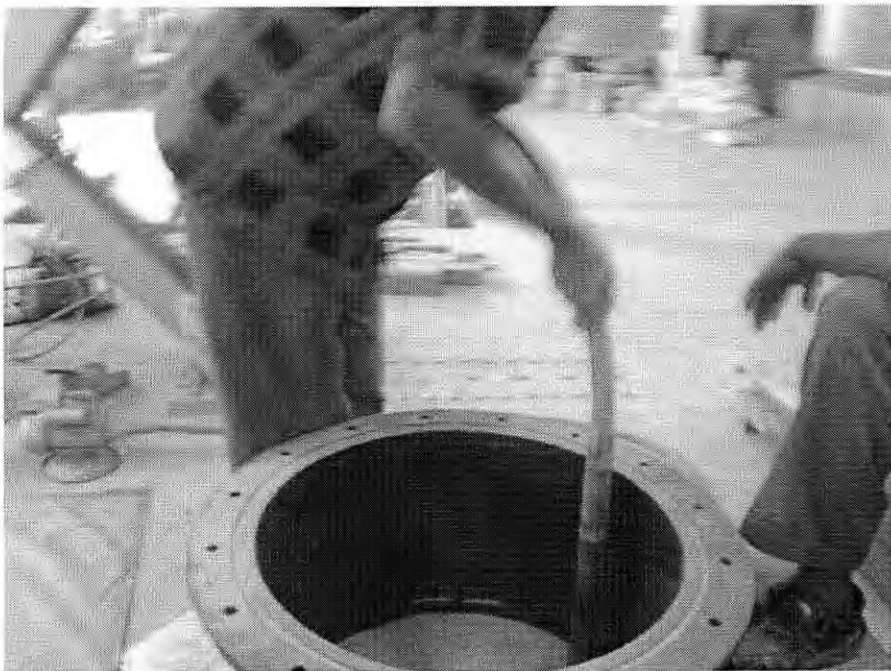
Fig. 3.12: Densification of sand into calibration chamber using concrete vibrator
