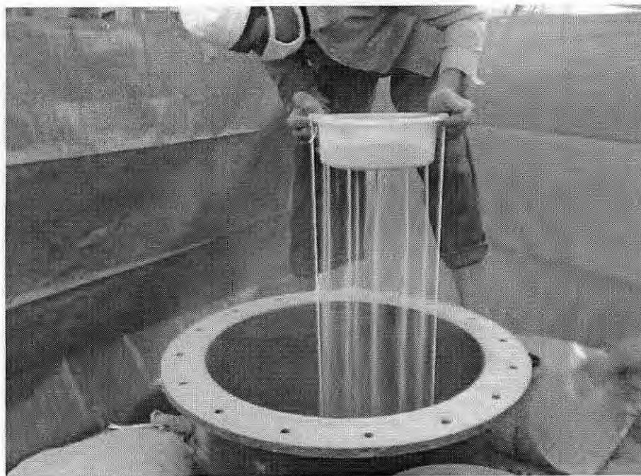
Fig. 3.9: Dry deposition into calibration chamber from discharging bowl maintaining a constant height of fall
