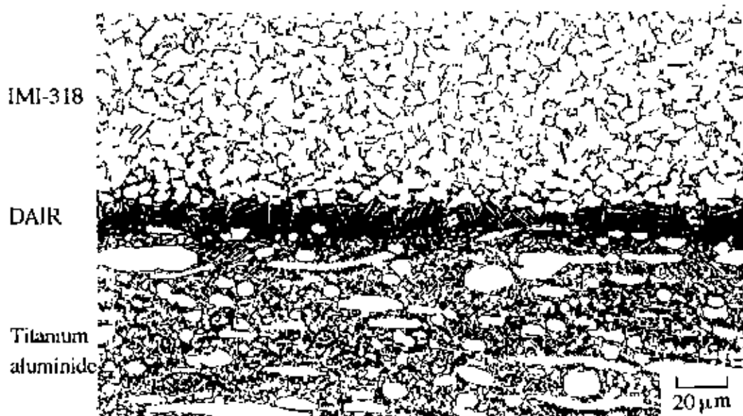
Figure 4.12 b - Microstructure of diffusion weld between IMI-318 to titanium aluminide using welding condition of 920°C + 10 MPa + 1 hr.
