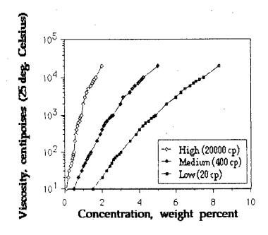
Figure 2.2.2: Sodium carboxymethyl cellulose: viscosity-concentration chart (Hercules Powder Co.). Viscosities in 2% solution in water at 25°C are shown in parentheses on the curves.
