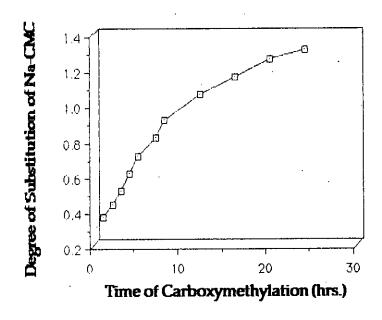
Figure 2.7.3. Variation of degree of substitution of Na-CMC with the time of reaction.
