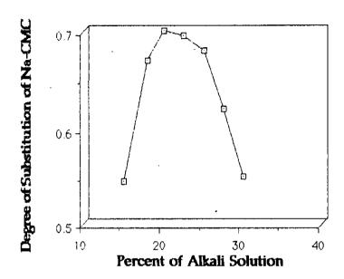
Figure 2.7.1. Variation of degree of substitution of Na-CMC with strength of alkali solution.
