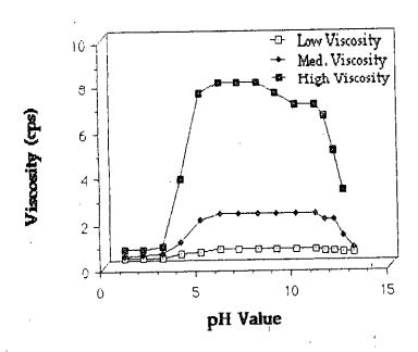
Figure 2.2.1. Carboxymethyl cellulose: variation of solution viscosity with pH (Brown & Houghton). Viscosities in 1% solution in water at 25 degrees Celsius.
