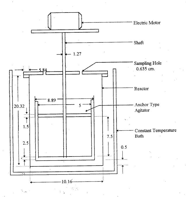
Figure 4.1.4. Diagram of the Reactor. (All dimensions in cm. Not upto scale)
