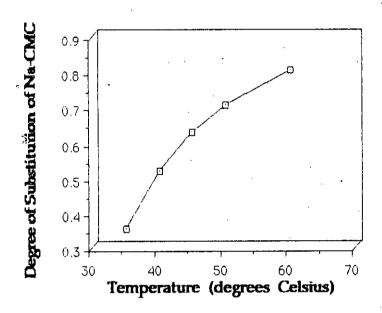
Figure 2.7.2. Variation of degree of substitution of Na-CMC with the temperature of reaction
