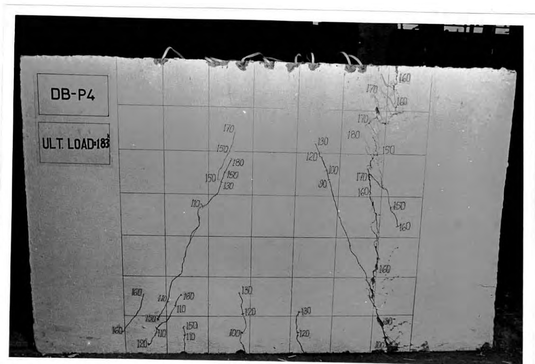
Fig. 5.22 Mode of Failure and Crack Pattern of Beam DB-P4
