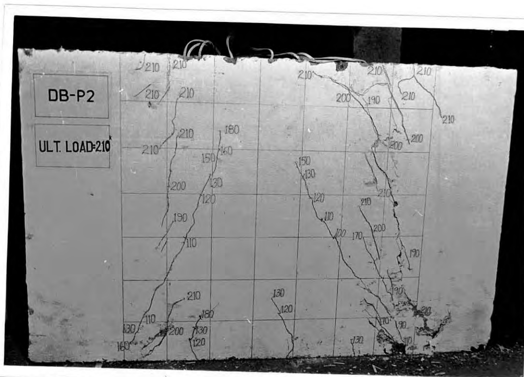
Fig. 5.20 Mode of Failure and Crack Pattern of Beam DB-P2
