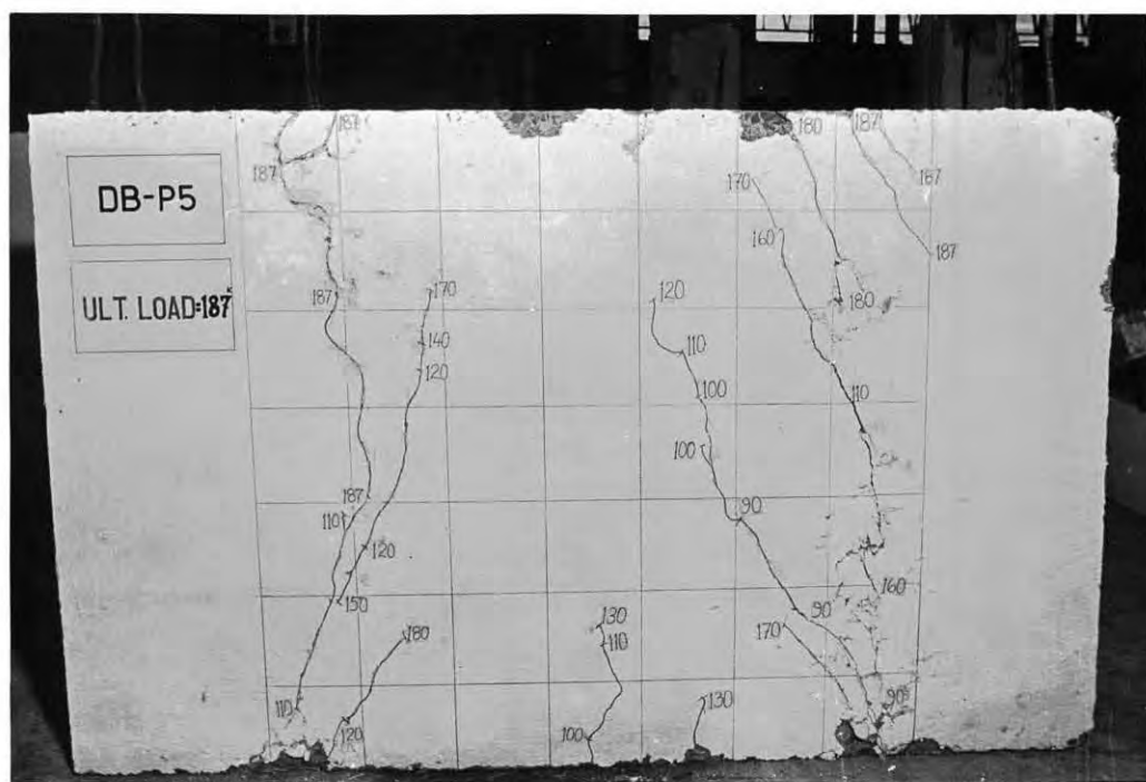
Fig. 5.23 Mode of Failure and Crack Pattern of Beam DB-P5
