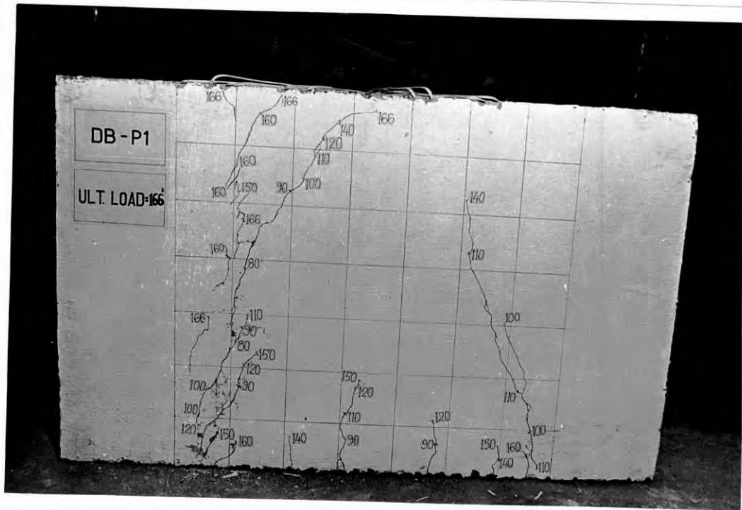
Fig. 5.19 Mode of Failure and Crack Pattern of Beam DB-P1
