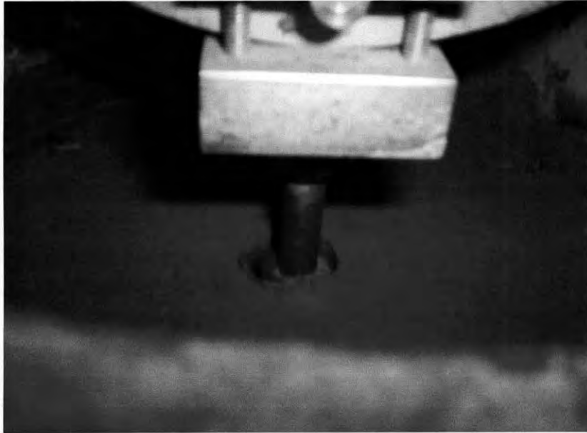
Fig. 9.1 Model scale footing on consolidation mold
