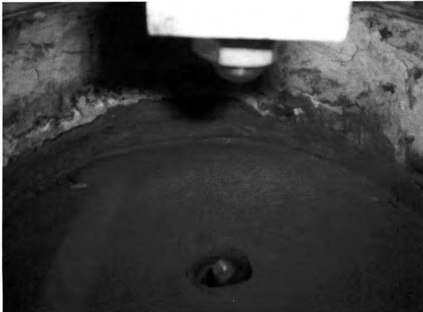
Fig. 9.2 Model scale footing on consolidation mold
