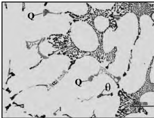
Figure 2.6.1: (1) Q-Al 5 Mg 8 Cu 2 Si 6 and (2) θ-CuAl 2 phases formed in an Al-Si-Mg alloy with 0.22% Cu [160]
