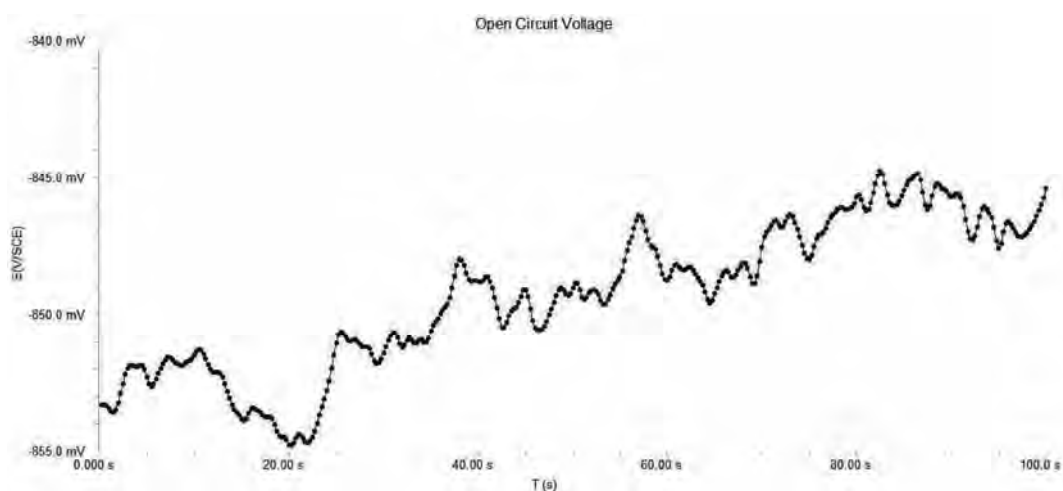
Figure 4.6.1: OCP variation with time for the peakaged Alloy-1 in 0.1M NaCl solution
