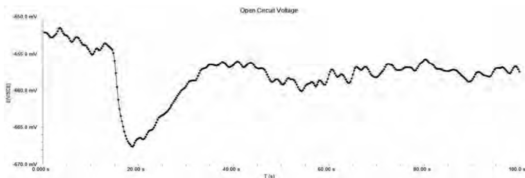
Figure 4.6.17: OCP variation with time for the peakaged Alloy-4 in 0.1M NaCl solution
