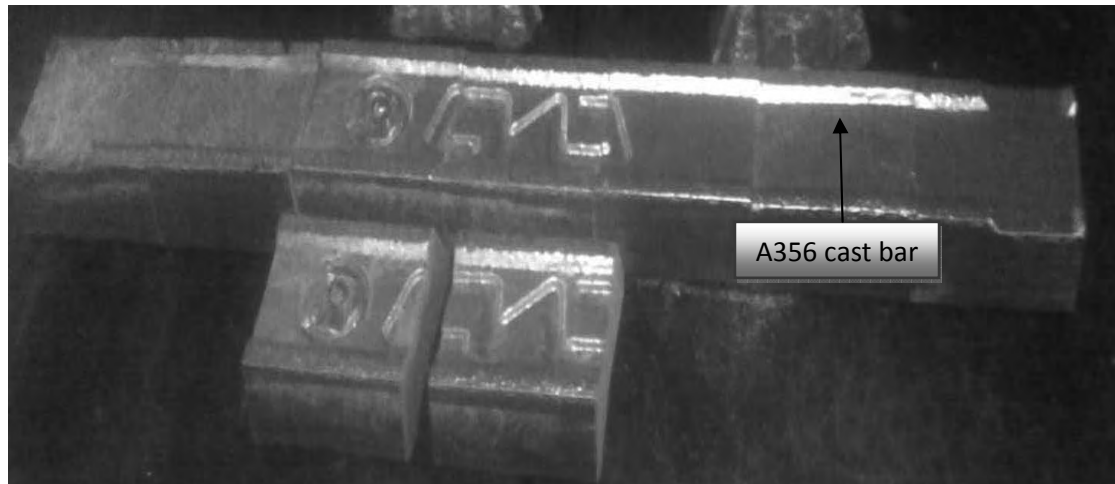
Figure 3.2.1: Photograph of an A356 ingot bar collected from WALTON with pieces prepared for further processing
