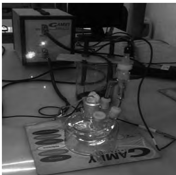
Figure 3.10.2: Gamry instrument set-up for electrochemical measurements
