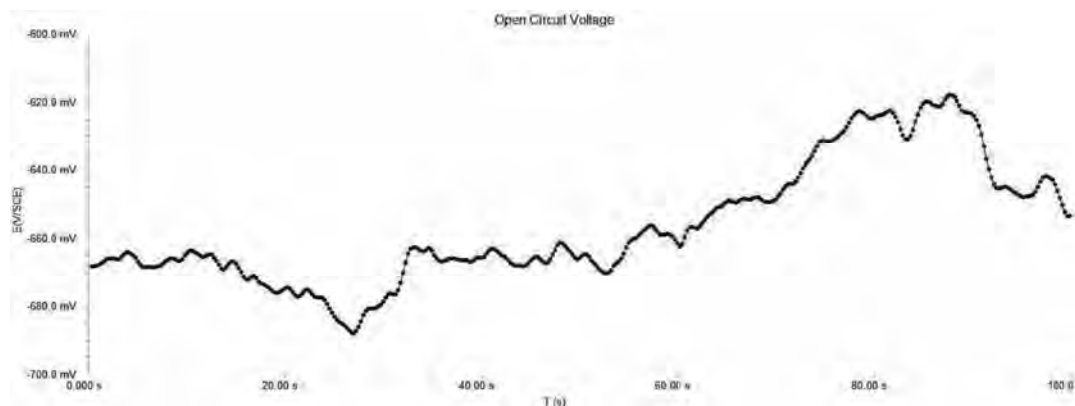
Figure 4.6.12: OCP variation with time for peakaged Alloy-3 in 0.1M NaCl solution
