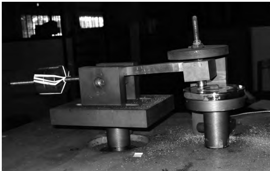
Figure 3.9.1: Pin-on-Disk type friction and wear test machine
