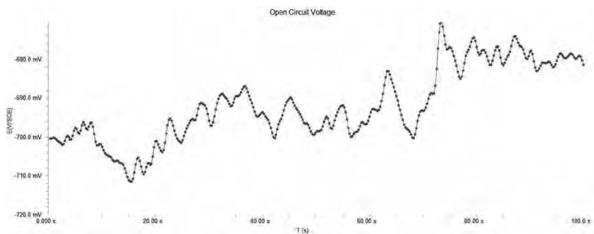
Figure 4.6.27: OCP variation with time for peakaged Alloy-6 in 0.1M NaCl solution
