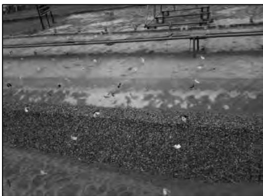
Figure A.45: Launching Behaviour of Stone Boulder
