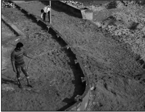
Figure A.17: Socking of Sand for Model Bed
