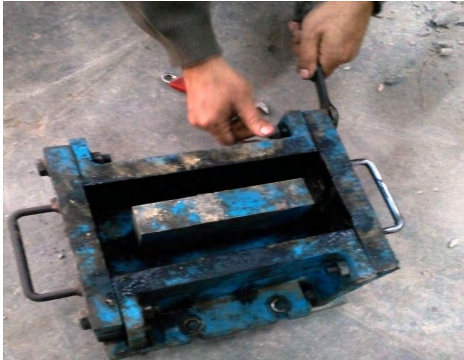
Figure 3.4: Mould and tightening of bolts.
