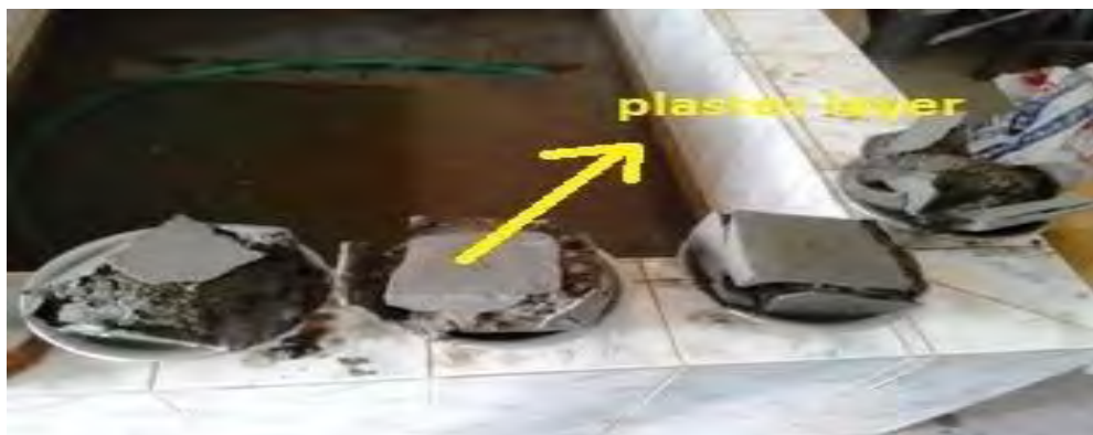
Figure 4.14: Plaster layer existing after 24 hours submergence under water.
