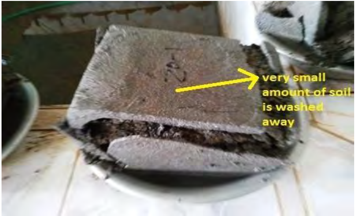
Figure 4.15: Photograph of CEB after absorption test.
