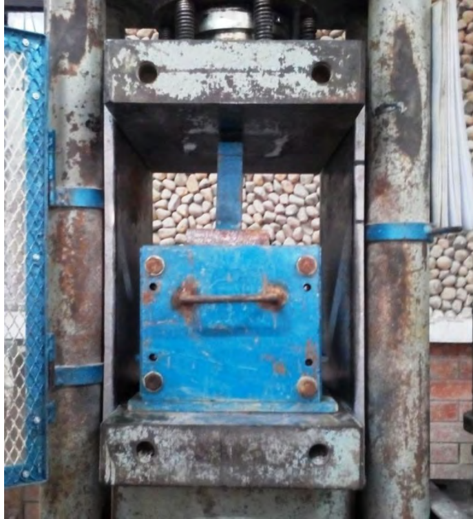
Figure 3.5: Mechanical press by compression testing machine.
