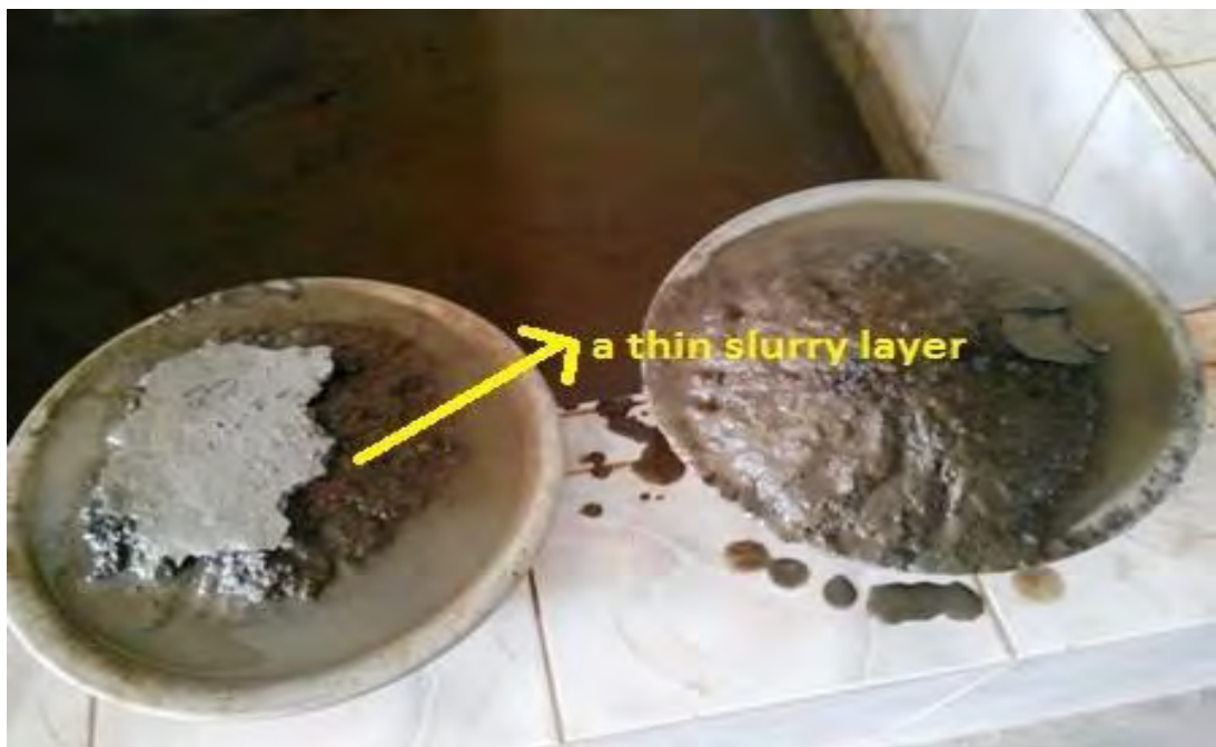
Figure 4.12: Photograph of CEB with slurry after 24 hours submergence under water.
