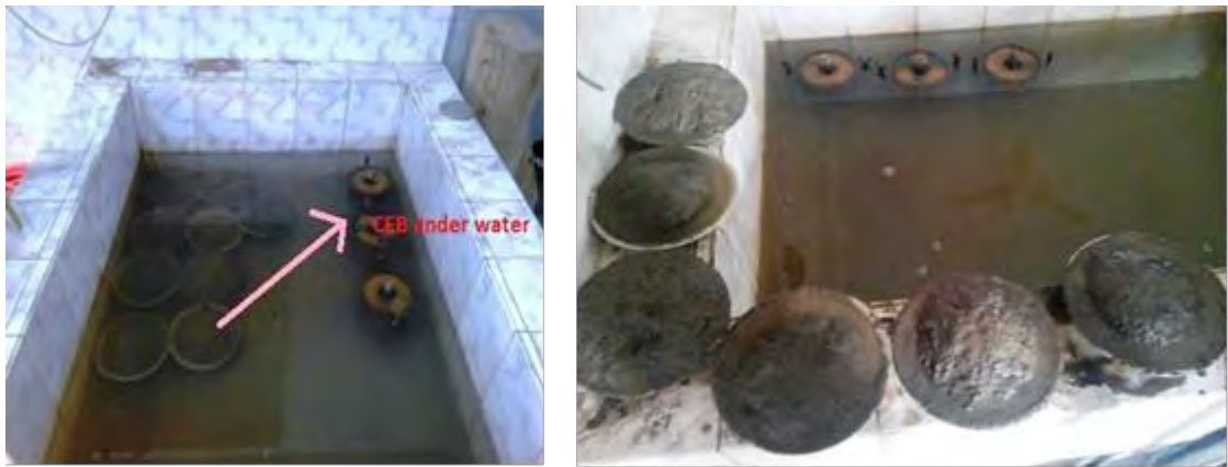
Figure 4.11: Photographs of (a) CEB under water; (b) after 24 hours.
