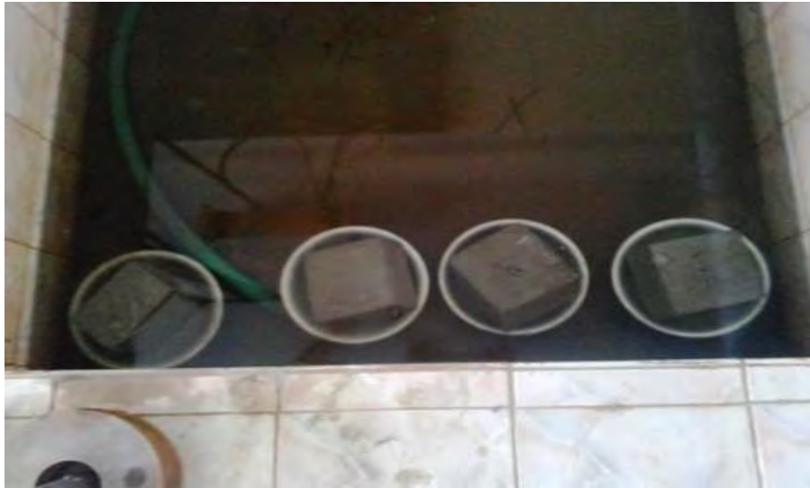
Figure 4.13: Photograph of CEB brick with plaster layer is under water.
