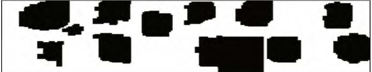
Figure 2.4: Binary masks of the TOBs are obtained using two consecutive morphological closing operations, first with line object L_5 and then with square object S_7 .
