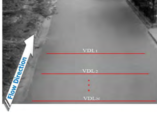
Figure 2.8: Frame showing a few number of VDLs perpendicular to the traffic flow
