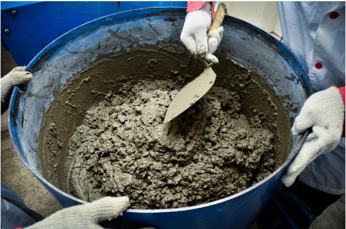
Figure 3.3: Concrete trial mix with sludge
