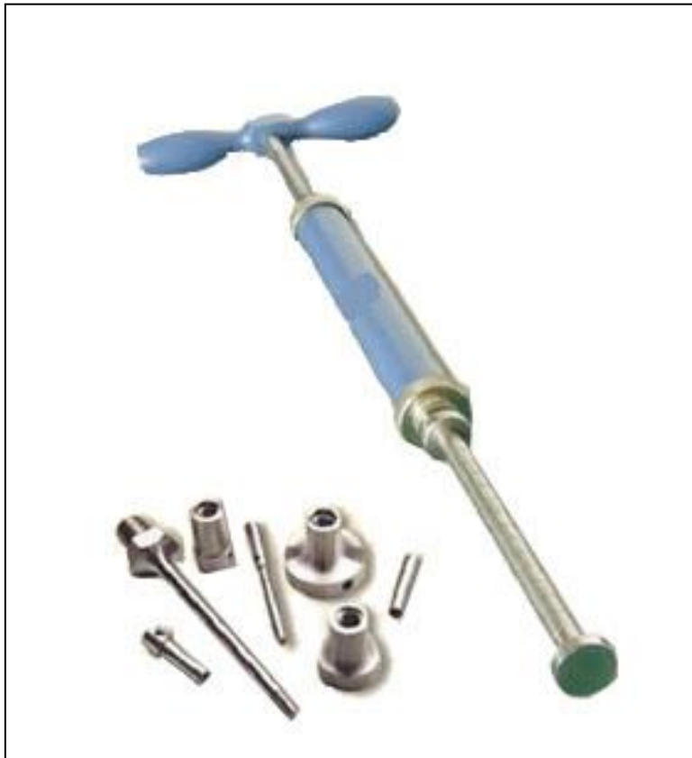
Figure 3.6: Concrete setting time measuring apparatus
