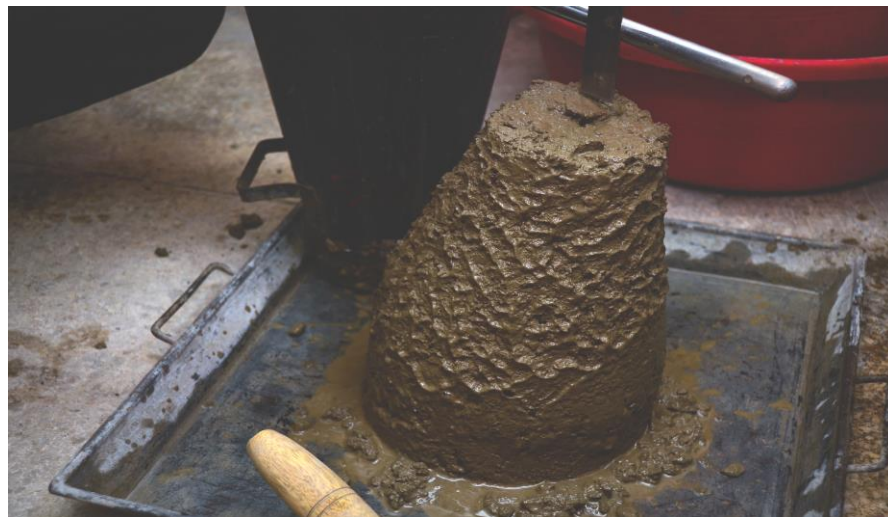
Figure 3.5: Measuring workability of the sludge mixed concrete
