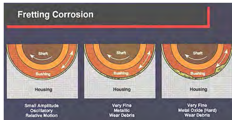
Fig. 2.23: Fretting corrosion wear [47]
