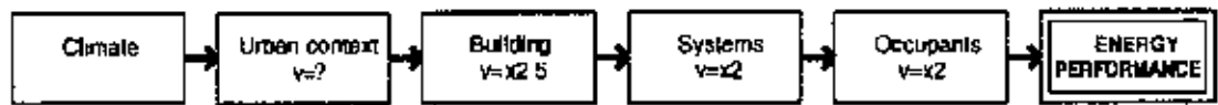
Figure 1.4: Factors that affect energy consumption in buildings; according to Baker and Steemers, 2000
