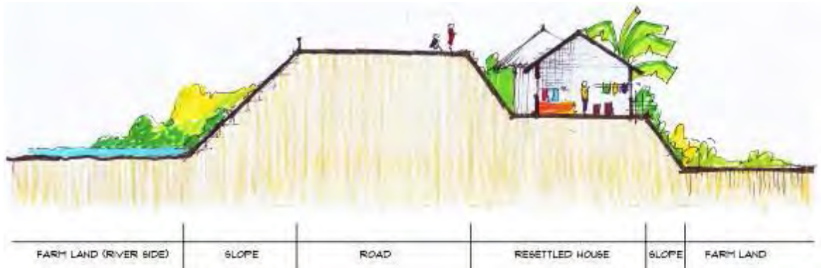
Figure 5.5: Section through the embankment shown the settlement on the down-slope of the embankment.
