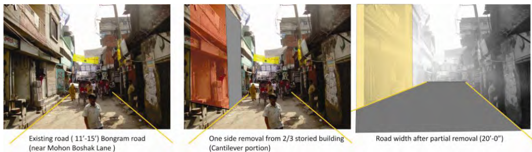
Figure 56: proposal for partial two or three storied building demolition for road widening (Bongram road)
