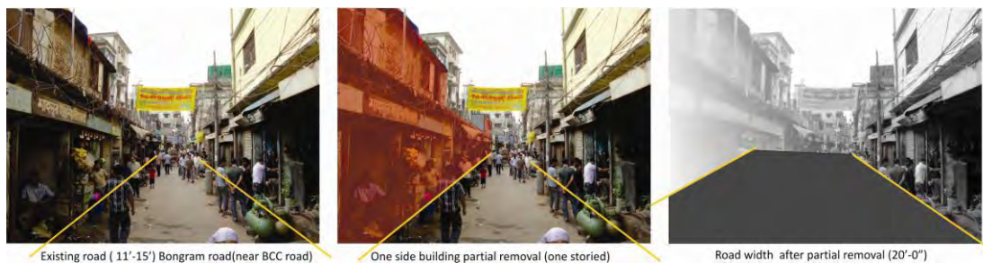
Figure 55: proposal for partial one storied building demolition for road widening (Bongram road)
