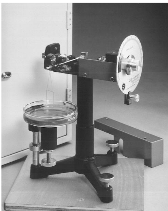
Fig. 3.7: Measurement of surface tension by DuNouy Ring Tensiometer.
