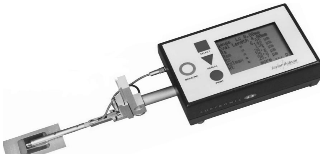
Fig. 3.6: Measurement of surface roughness by Surtronic 25 roughness checker.
