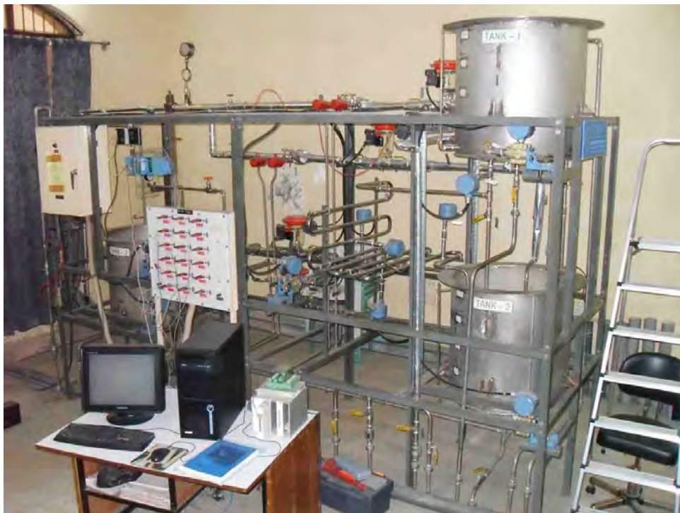
FIGURE 4.2: Experimental setup of a two tank pilot plant heating system
