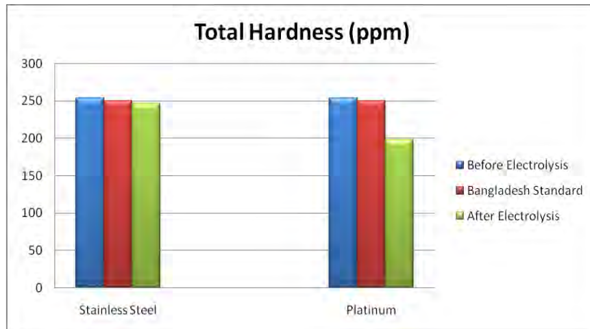
Fig 3.10 Total Hardness of tap water with the variation of electrode using 5 Volt potential, NaCl as electrolyte and 1 Hr as contact time
