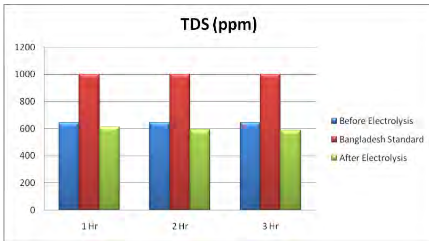
Fig 3.16 Total Dissolved Solid of tape water with the variation of time using platinum electrode, 5 Volt potential and NaCl as electrolyte
