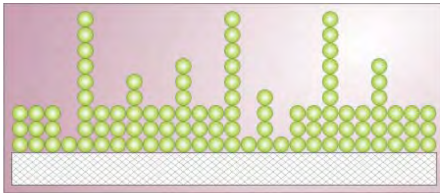
Figure 1.11: Brunauer's model of multilayer adsorption, that is, a random distribution of sites covered by one, two, three, etc., adsorbate molecules 2 .
