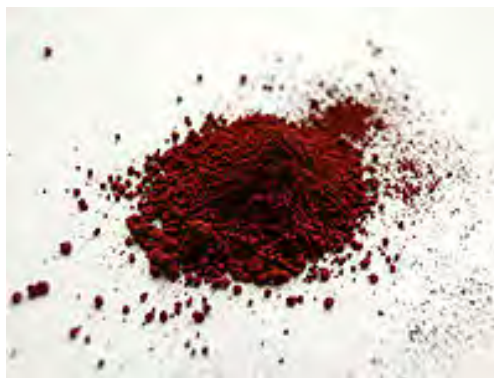
Figure 2.2 (c) : Photo of the prepared iron oxide
