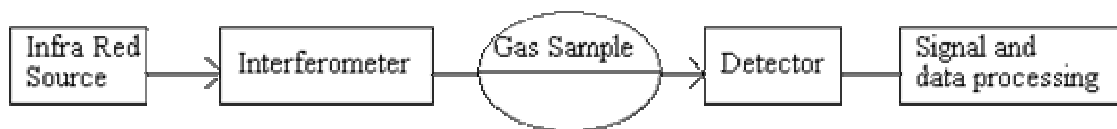
Figure 1.19: Basic components of FT-IR 76(a)
