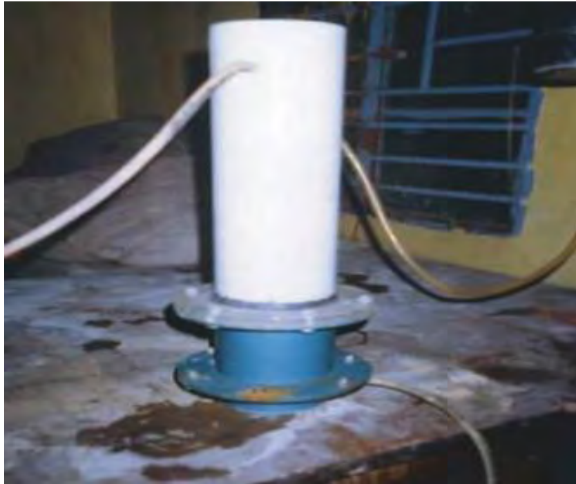
Figure 2.15 Permeameter for geojute-soil system (after Sarma 2005)
