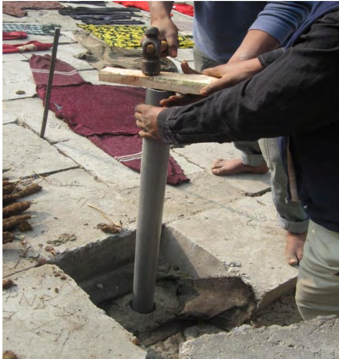
Figure 3.5 Collection of soil sample through PVC pipe
